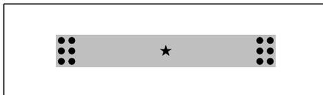
Fig. 3. The shaded rectangle corresponds to the cell shape of a right or left moving cell in our model for rippling. This cell is  $3 \times 21$  nodes for a  $1 \times 7$  aspect ratio. The star in this figure corresponds to the cell's center and the nodes of the interaction neighborhood where C-factor is exchanged are indicated by black squares at the cell poles.
