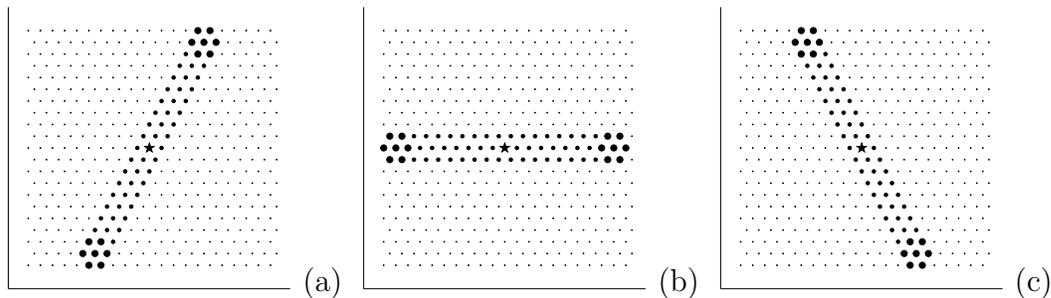
Fig. 9. The cell shapes of a) a cell oriented 60 or 240 degrees, b) a cell oriented 0 or 180 degrees and c) a cell oriented 120 or 300 degrees. All cells are  $3 \times 21$  for a  $1 \times 7$  aspect ratio. Each cell’s “center of mass” is indicated by a star and the nodes of the interaction neighborhood where C-factor is exchanged are indicated by the larger black disks at the cell poles.
