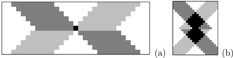
Fig. 6. Space-time plot of a wave inter-penetration. Time increases as the vertical axis descends. Right-directed particles are shown in dark gray, left-directed particles are shown in light gray. a) Phase jump of one cell length (9 units) as two cells collide and immediately reverse. b) Phase delay as two cells collide and travel 8 time-steps before reversing.
