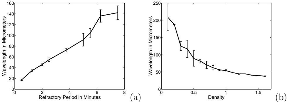
Fig. 5. a) Average wavelength in micrometers versus refractory period in minutes. Cell length  $\ell = 4$ ,  $\delta = 1$ . The internal timer is adjusted so that the fraction of clock time spent in the refractory period is constant:  $t = 3R/2$  and  $\tau = 5 * R/2$ . b) Average wavelength in micrometers versus density (total cell area over total lattice area). Cell length = 4 with an internal timer given by  $R = 8$ ,  $t = 12$ ,  $\tau = 20$ .
