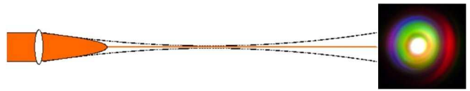
FIG. 1 Principle of producing femtosecond filaments in air at the laser wavelength of 800 nm. Photograph at the right-hand side shows a transverse cut of the filament profile.
