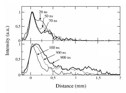
Figure 4: Intensity profiles recorded during ablation of Ti in 500 Pa He with  $F_{las} = 3 \text{ Jcm}^{-2}$  using the fundamental wavelength at  $\lambda = 800 \text{ nm}$ .
