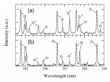
Figure 8: Optical emission spectra recorded during ablation of Zr in 500 Pa He with  $F_{las} = 3.0 \text{ Jcm}^{-2}$  ( $\lambda_{las} = 800 \text{ nm}$ ) for t = 50 (a) and 70 ns (b) and  $z = 150 \mu\text{m}$ .
