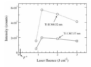
Figure 13 : Spectral line emission intensities of ions and neutral atoms as a function of  $F_{las}$  for Ti ablation in 500 Pa He at  $\lambda_{las} = 800$  nm.
