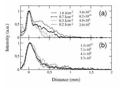
Figure 6: Intensity profiles recorded for different laser fluences for t = 20 (a) and 400 ns (b) during ablation of Ti in 500 Pa He with  $\lambda_{las} = 400$  nm.
