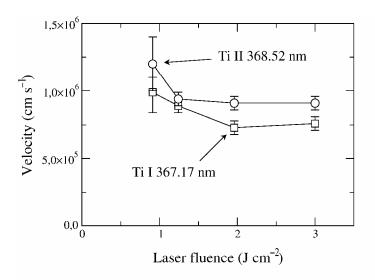
Figure 12: Propagation velocities of neutral atoms and ions as a function of  $F_{las}$  observed during Ti ablation in 500 Pa He using  $\lambda_{las} = 800$  nm.
