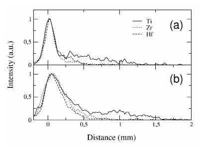
Figure 7: Intensity profiles recorded during ablation of Ti, Zr and Hf for t = 100 (a) and 900 ns (b) in 500 Pa He with  $F_{las} = 1.6 \, \mathrm{Jcm}^{-2}$  and  $\lambda_{las} = 400 \, \mathrm{nm}$ .
