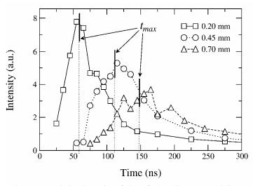
Figure 9: Emission intensity of the Hf I 417.43 nm spectral line as a function of time for different distances from target. The recordings correspond to ablation of Hf in 500 Pa He with  $F_{las} = 3.0 \, \mathrm{Jcm^{-2}}$  ( $\lambda_{las} = 800 \, \mathrm{nm}$ ).
