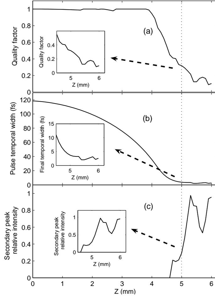
FIG. 4: (a) Quality factor, (b) temporal width, and (c) relative intensity of the secondary peak as a function of propagation distance inside the PCF for the same initial pulse of figure 3. The dotted vertical line denotes the fiber length.
