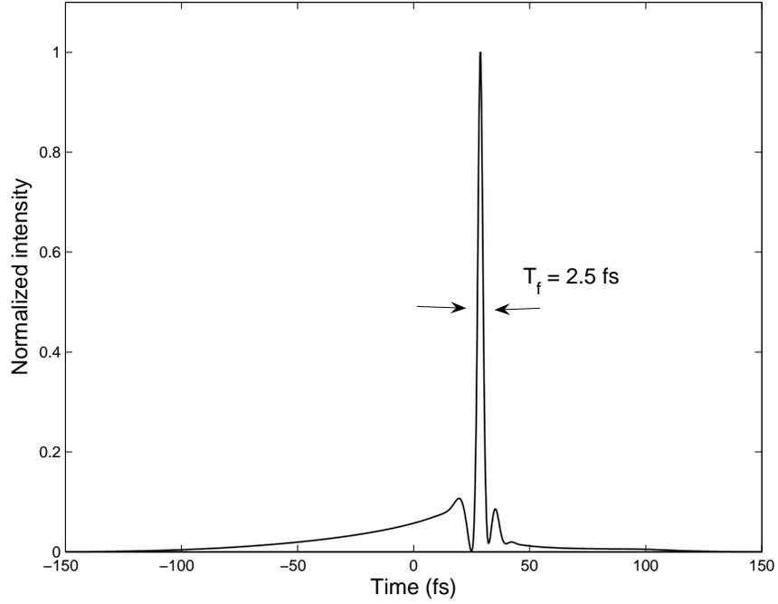
FIG. 6: Single-cycle pulse obtained for the same initial pulse of figures 3 and 4, in the hypothesis of a *completely* flat dispersion profile, i.e.  $\beta(\omega) \simeq 1/2\beta_2(\omega_0)(\omega - \omega_0)^2$ .
