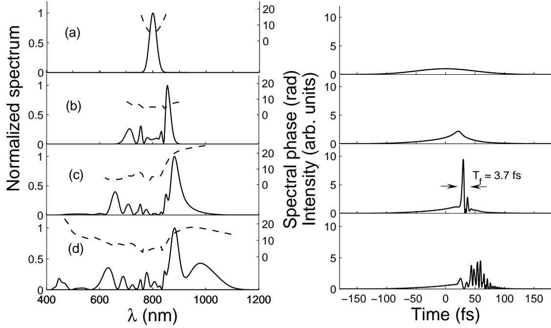
FIG. 3: Spectra, spectral phases, and temporal profiles corresponding to (a)  $z = 0$ , (b)  $z = 4$  mm, (c)  $z = 5$  mm, (d)  $z = 6$  mm for a 30 fs laser pulse of initial energy  $E = 5 \times 10^{-10}$  J that has been temporally broadened to 119 fs.
