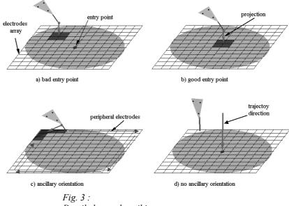
Detailed area describing : a), b): tip code and c), d): orientation code example. rigid bodies: one mounted on a surgical tool and the other one used as a reference, to calculate, in real time, the position and transformations of the two points previously calibrated. This information, corresponding to position and orientation of surgical instrument, is with pre-planned compared the trajectory to measure errors and is coded to use it as feedback information to the interfaceable strip.
