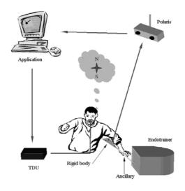
*Fig. 1: Configuration of the system*
