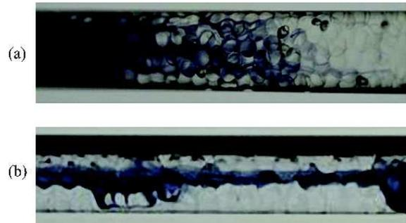
FIG. 6: Miscible displacements of pure glycerol by dyed glycerol saturating disordered glass beads packings inside a  $D = 8$  mm diameter capillary tube. Bead diameter : (a)  $d = 2$  mm - (b)  $d = 3$  mm. The tube/particle diameter ratio is respectively 4 and 2.66.
