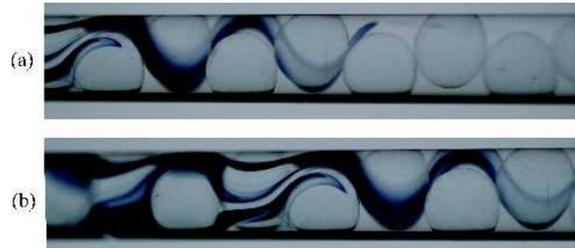
FIG. 7: Views at different times of the miscible displacement front of pure by dyed glycerol in a disordered channel: the diameter of the beads is  $d = 6$  mm and the diameter of the tube  $D = 8$  mm. The tube-to-particle ratio is 1.33.
