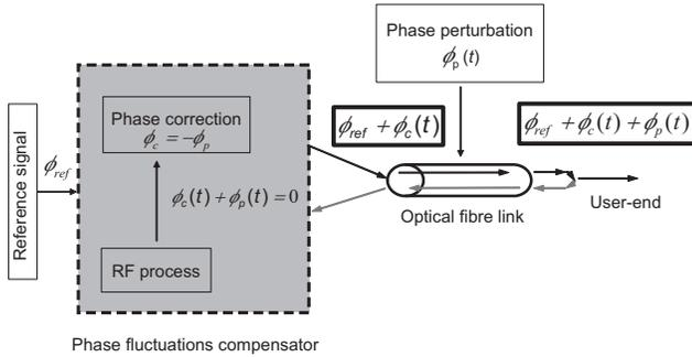
Figure 3: Schematic of the phase fluctuations compensation
