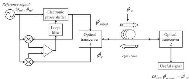
Figure 4: Simplified schematic of the phase conjugator
