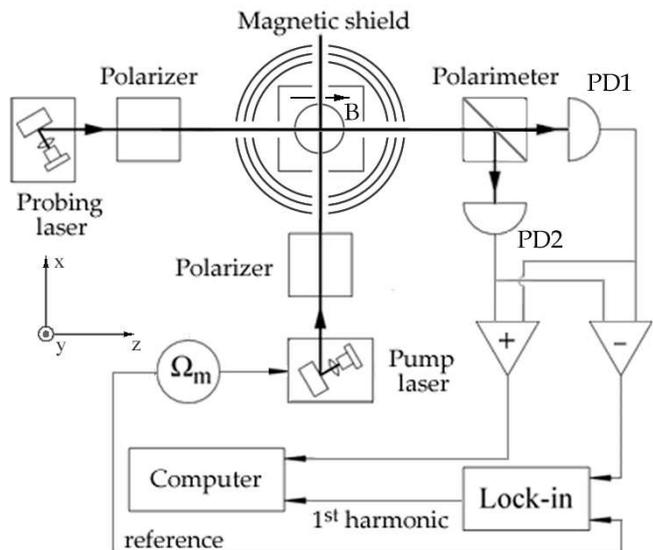
FIG. 3: Experimental setup. PD1 and PD2 are photodiodes.
