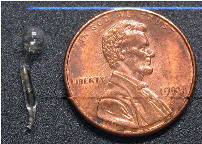
FIG. 1: Cs-vapor microcell, whose inner walls are coated with paraffin, used for the present measurements.
