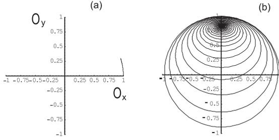
**Figure 6.** Evolution of polarization toward stationary solution in the case  $\mathbf{r} = \{0.01, 0, 0.3\}$ ,  $\mathbf{h} = \{1, 0, 0\}$ , (a) and when  $\mathbf{r} = \{0.01, 0, 1.2\}$ ,  $\mathbf{h} = \{1, 0, 0\}$  (b)
