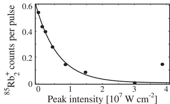
FIG. 2:  $^{85}\text{Rb}_2^+$  counts per ionization pulse vs. peak intensity of the applied fs pulses (filled circles). Each data point represents the accumulated result of an identical number of ionization laser shots. An exponential decay fit of the data is shown (solid line).
