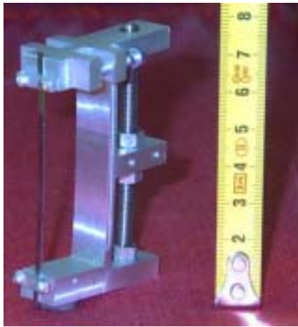
Figure 8: The implemented structure for bending crystal strips.
