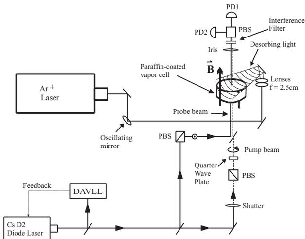
FIG. 3: Schematic diagram of the experimental setup. PBS - polarizing beamsplitting cube, PD1(2) - photodiodes for light detection in polarimeter, DAVLL - Dichroic Atomic Vapor Laser Lock (described in text and shown in Fig. 4).
