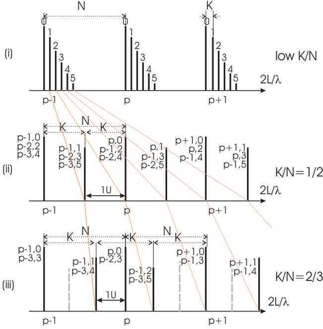
FIG. 1: partial transverse and longitudinal comb in 3 configurations. (i) low  $K/N$  cavity (ii) cavity with  $K/N=1/2$ , for instance confocal (iii) cavity with  $K/N=2/3$ .  $K$  and  $N$  are integers. for (ii) and (iii) we indicated besides each peak the first possible modes  $(p, s)$ . For simplicity sake, we represented on (iii) the peaks corresponding to other combs with grey dashed line.
