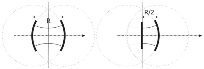
FIG. 3: The confocal cavity (left) has a symmetry plane. Placing a plane mirror in this plane gives us the hemi-confocal cavity (right).
