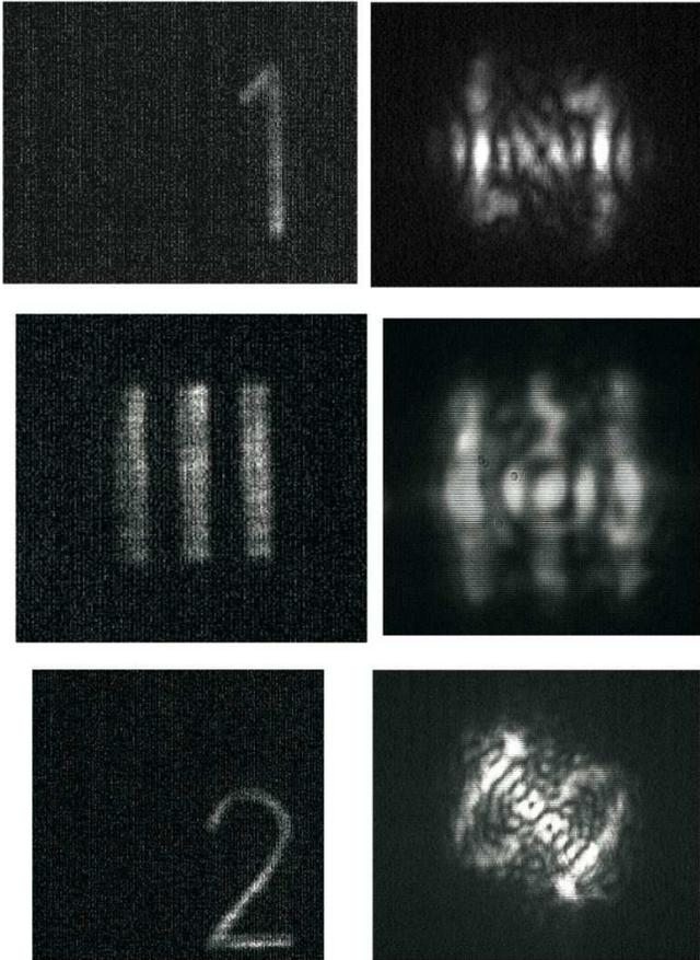
FIG. 10: Image on the resolution target (left) and their transmission through the hemi-confocal cavity (right).
