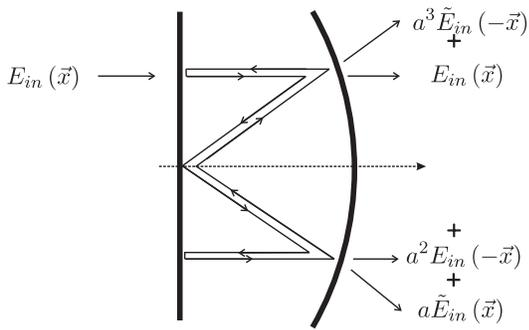
FIG. 4: Ray trajectory picture in the hemi-confocal cavity
