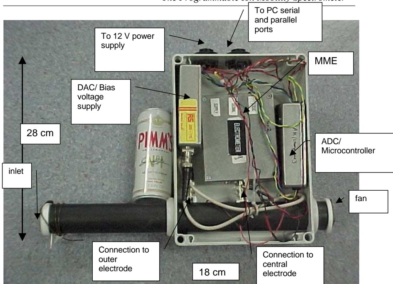
Figure 5.17 Photograph of the PIMS ready for atmospheric deployment (without lid on box).
