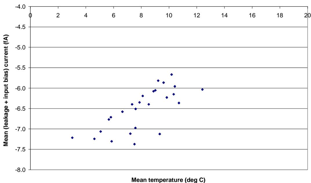
Figure 3.7 Daily mean leakage current and temperature for March 1998, calculated from automatically logged five minute averages of capped current amplifier output (in volts) and temperature.
