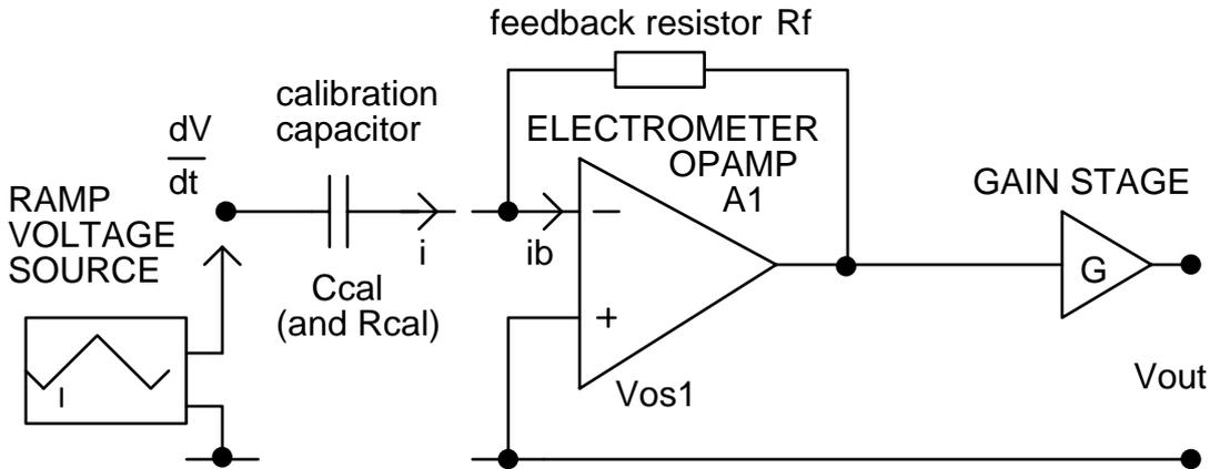
Figure B.2 Capacitive generation of calibration current  $i$ .
