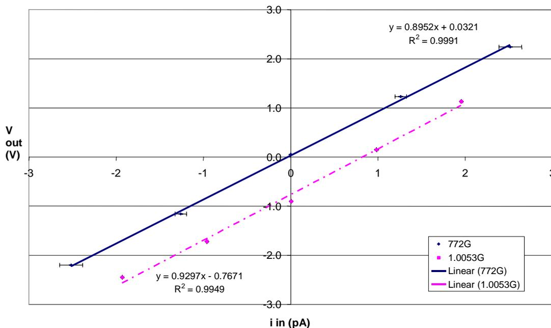
Figure 5.10 Resistive calibration of the MME in picoammeter mode, using calibration resistors of 772 GΩ and 1 GΩ. The error bars on the abscissa result from the uncertainty in the magnitude of the calibration resistor.
