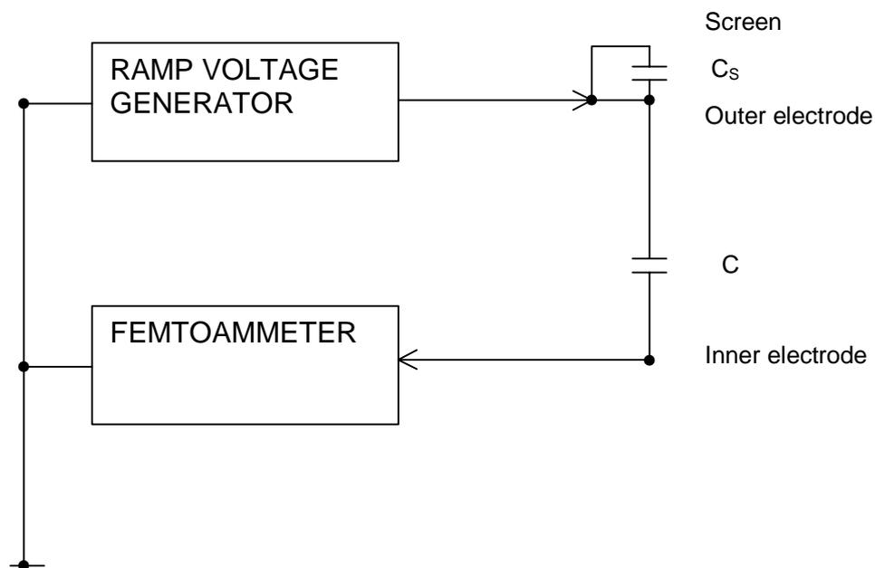
Figure 5.16 Schematic of the circuit used to measure the Gerdien capacitance.
