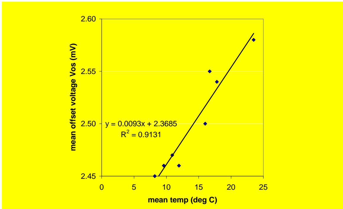
Figure 5.12 Variation of mean input offset voltage of the MME with mean temperature, over eight diurnal cycles.
