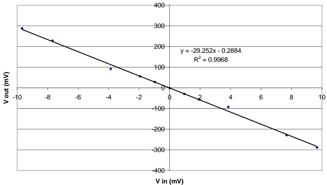
Figure 5.9 Direct calibration of the second gain stage, with  $V_{in}$  applied at the input to the gain stage (with first op-amp disconnected) and  $V_{out}$  measured at the electrometer output.
