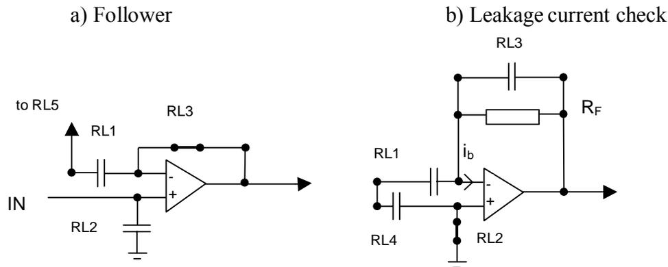
Figure 6.10 Differences between the MME follower and leakage current measurement configurations a) and b). In this simplified diagram, an open relay is represented as a capacitor, as it transiently injects charges when opening, and a closed relay (thick line) is a direct connection.
