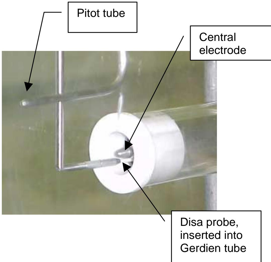
*Figure 3.9 Photograph of the Disa probe inserted into the end of the Gerdien, and showing the Pitot tube which measured the external flow.*
