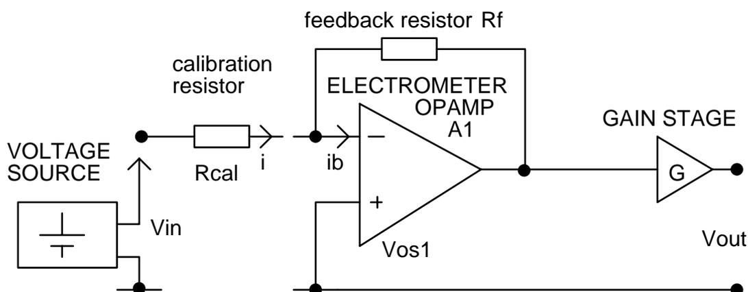
Figure B.1 Resistive generation of calibration current  $i$ .
