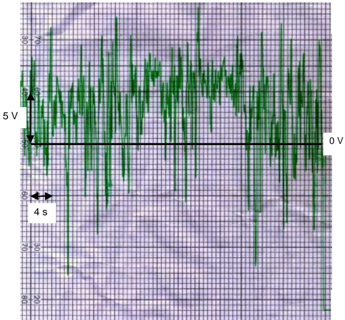
Figure 6.15 Sample of the Arizona Gerdien output at  $V_b = -105$  V. The chart recorder trace is centred at 0 V, and axis scaling is indicated on the trace.
