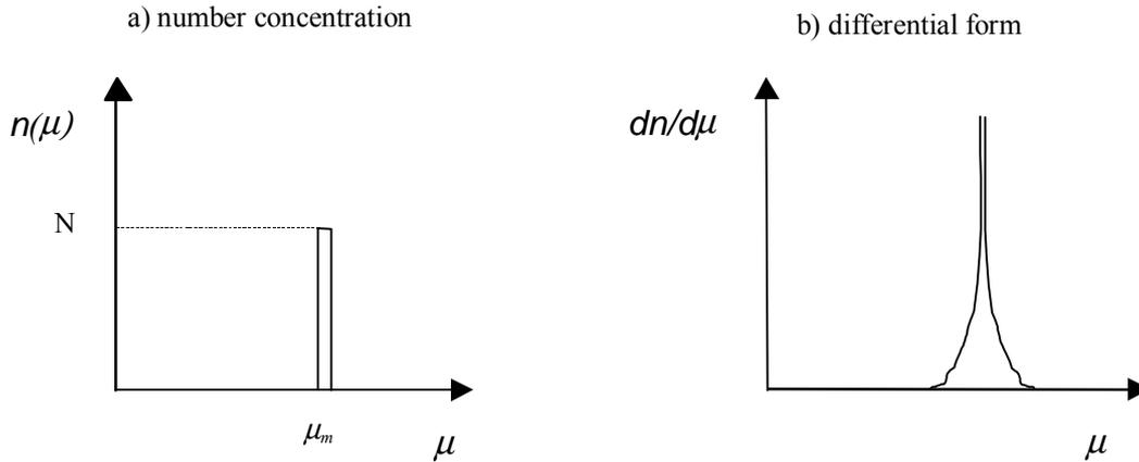
Figure 8.1 a) The simplest ion mobility spectrum: unimodal, when all ions have the same mobility. b) is the same spectrum expressed in differential form.
