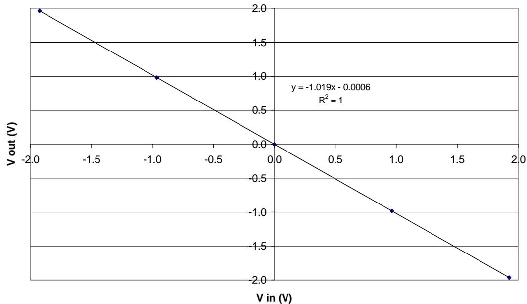
Figure 5.8 Calibration of the voltage follower mode, for  $V_{in}$  applied at the input, and  $V_{out}$  measured at the electrometer output.
