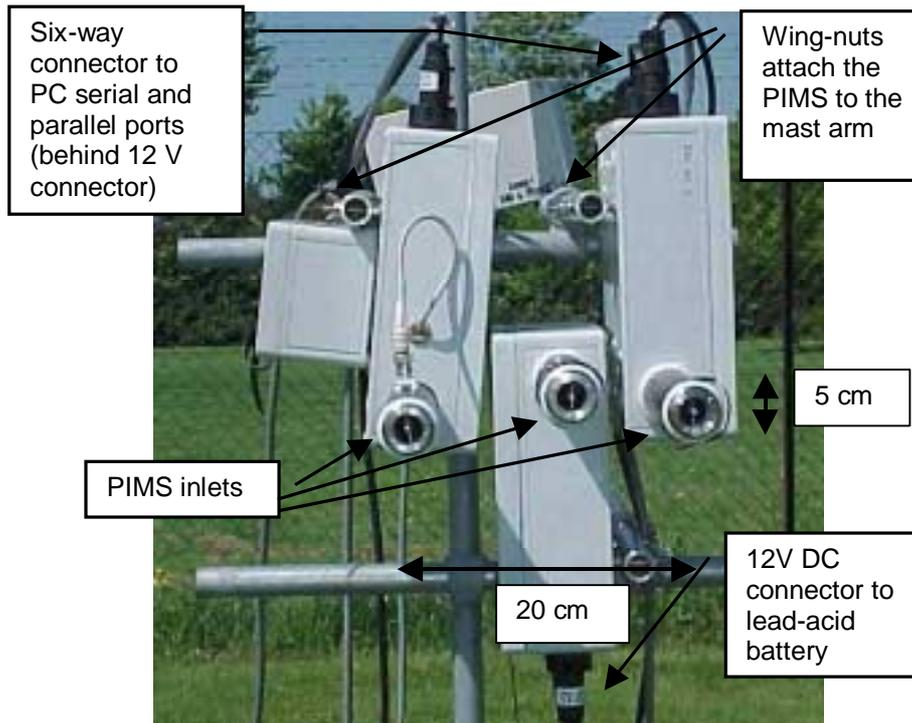
Figure 6.3 Close-up photograph, taken from the south, showing the PIMS inlets and connections.
