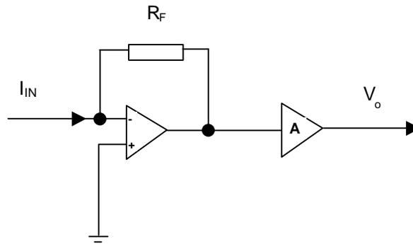
Figure 3.5 Feedback current amplifier including gain stage *A*
