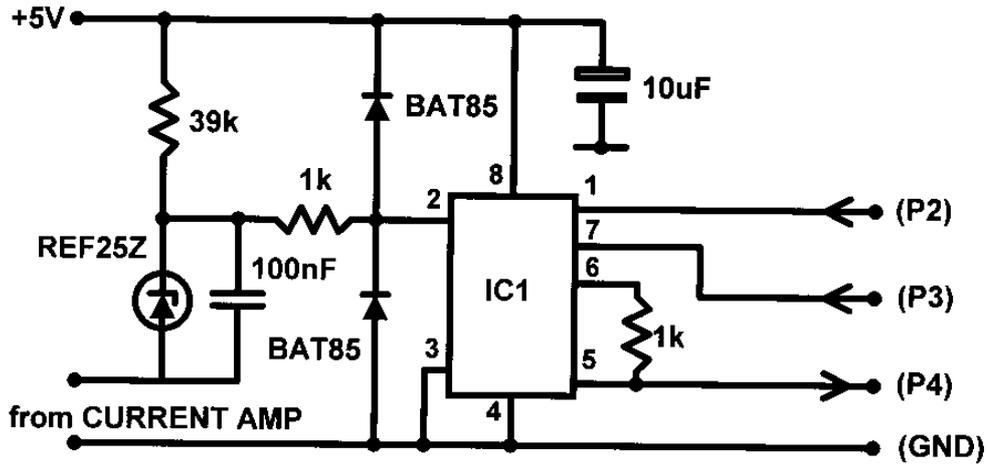
Figure 4.2 Schematic diagram of the ADC (IC1) and level-shifting circuitry, showing the power supply and connections to the microcontroller I/O pins. From Aplin and Harrison (2000).
