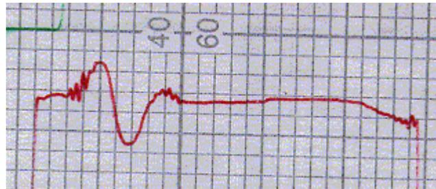
Figure 3.14 Example of the oscillations in the current amplifier output ( $C_G \sim 8\text{ pF}$ ) when subjected to a step change from 100 to 200 fA. Oscillations are clearly visible each time a transient is induced. The x-axis scaling is 1 small square = 0.2 s. y-axis scaling is approximately 4 mV/small square (the total amplitude of the oscillation was about 10 % of the signal)
