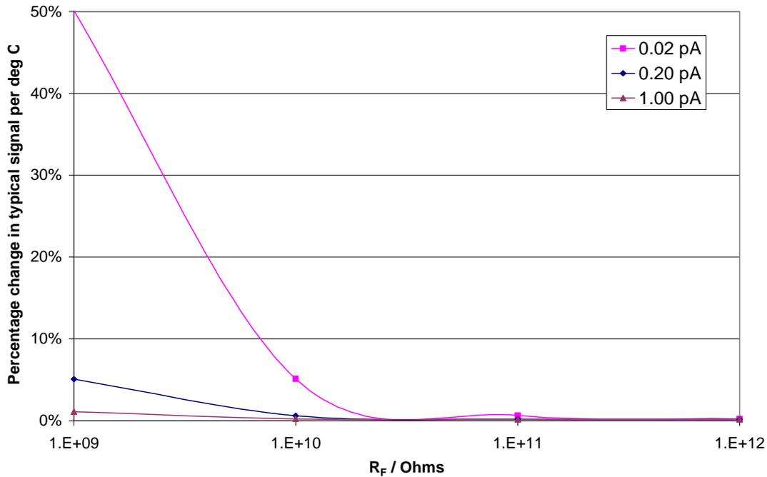
Figure 3.6 Temperature sensitivity of the output voltage with  $R_f$  for typical input currents from atmospheric ions (shown in pA in the legend), calculated from Eq. 3.9.
