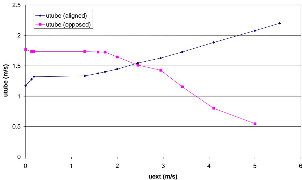
Figure 3.10 Relationship between the flow in the tube  $u_{\text{tube}}$  and the external ventilation  $u_{\text{ext}}$ , for the two cases where the external and fan flow are in the same and opposite directions.
