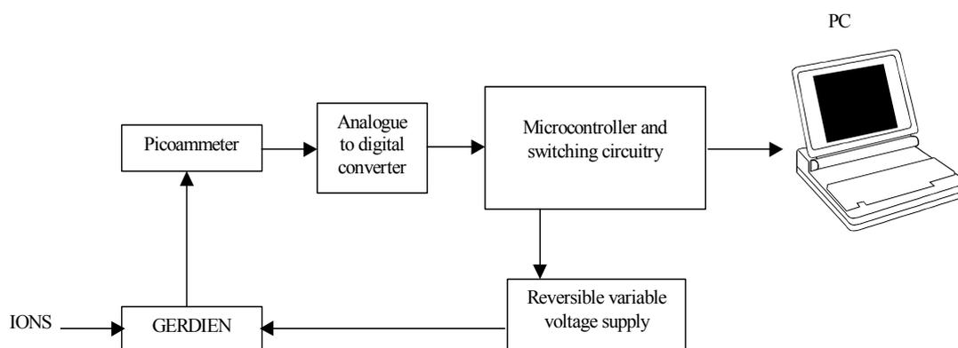
Figure 4.1 Schematic showing the integrated air ion measurement system, from Aplin and Harrison (1999)
