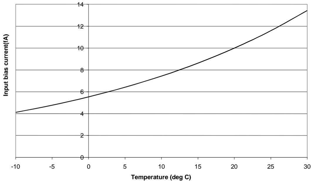
Figure 3.8 Variation of the typical MAX406 input bias current with temperature (from manufacturer's data sheet).
