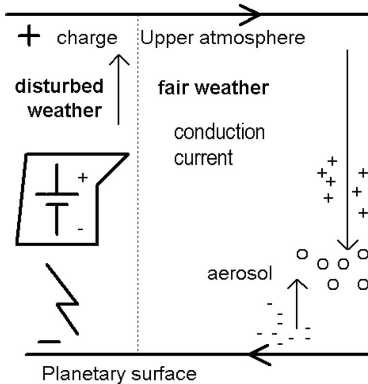
Figure 1.3 The global atmospheric electrical circuit (Harrison and Aplin, 2001) showing the combination of charge separation from thunderstorms, and maintenance of the circuit by air ions.
