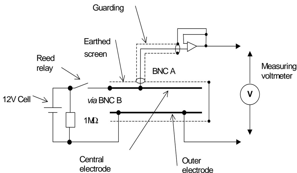
Figure 3.19 Voltage Decay measurement configuration. The  $1M\Omega$  resistor in the reed relay part of the circuit was needed to protect from transients. The cell supplies the bias voltage to the electrodes, controlled by the relay.
