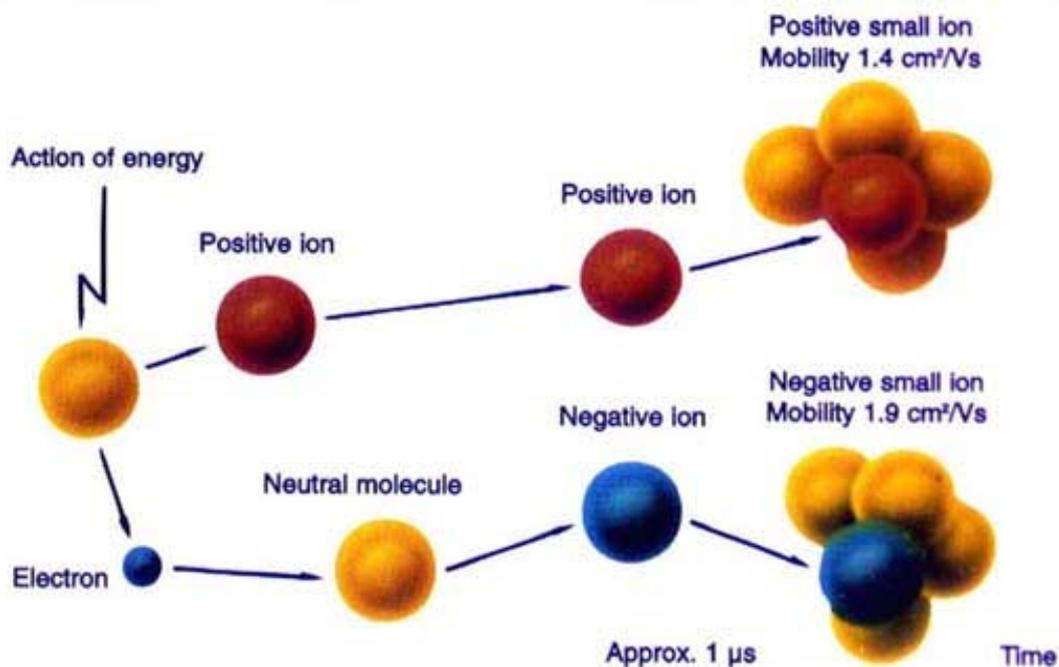
Figure 1.1 Schematic illustrating the production of atmospheric small ions from neutral molecules.
