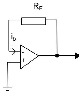
Figure 5.5 Schematics for measurement of a) input offset voltage  $V_{os}$  b) leakage current. (Power supplies are omitted for clarity)
