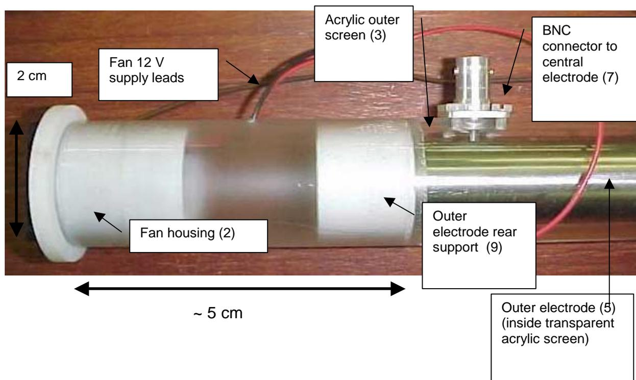
Figure 5.2 Photograph of one end of the partially constructed new Gerdien tube, before the conducting tape over the acrylic outer screen has been added. (The fan is in place and can just be seen to the left of the fan housing).
