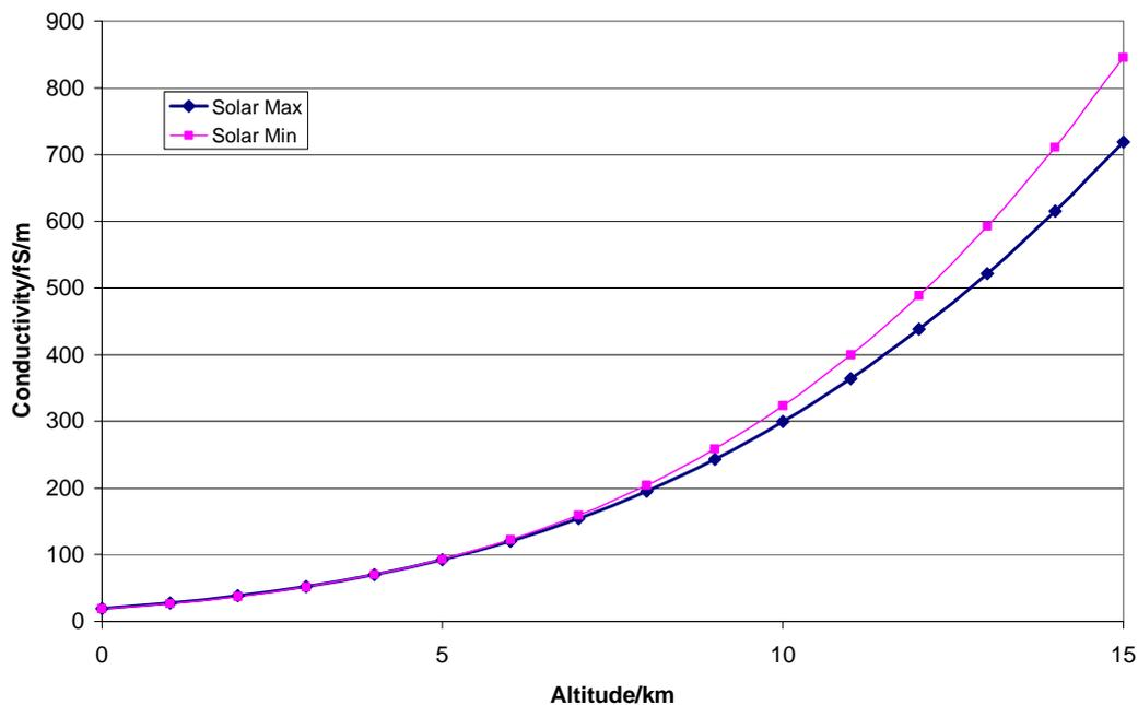
Figure 2.6 Variation of positive conductivity with altitude and solar cycle, calculated using Eq. 2.23 from Gringel (1978).
