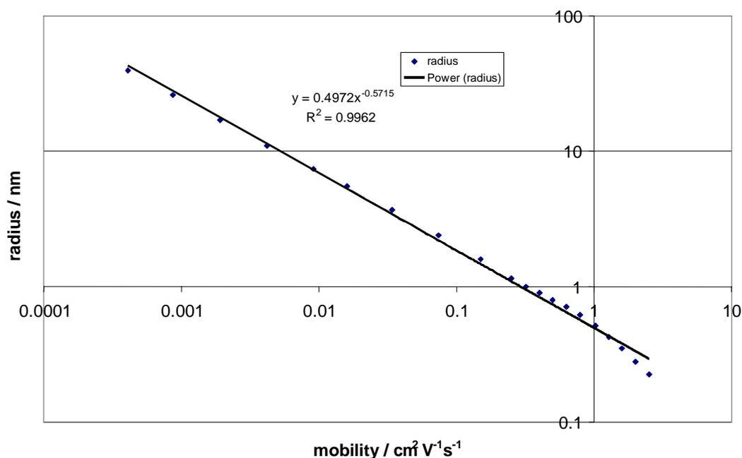
Figure 3.11 Relationship between ionic mobility and radius, originally calculated using Tammet's (1995) expression and here reduced to a simple power law.
