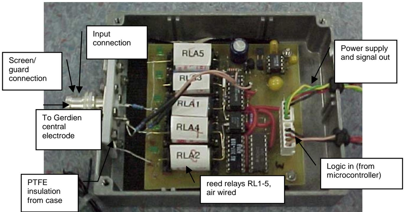
Figure 5.7 Photograph of the multimode electrometer.
