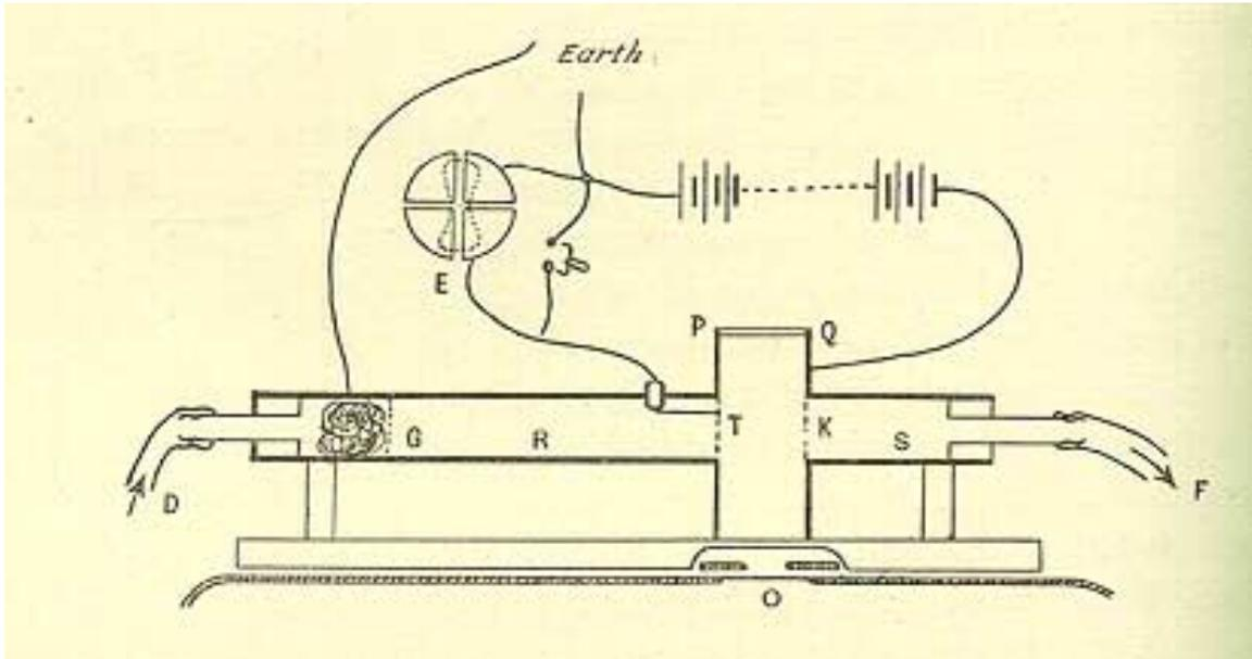
Figure 2.1 The apparatus used by Zeleny to measure ionic mobility. The gases enter at D, pass through a plug of wire wool, to remove “dust”, and leave at F. O is an ionising X-ray source. Q and P are brass plates with a voltage across them. T and K are wire gauze. If the ions produced hit P, Q or K they are conducted to earth, but ions hitting T modify its potential, which is measured relative to the battery by the electrometer E (Thomson, 1928).
