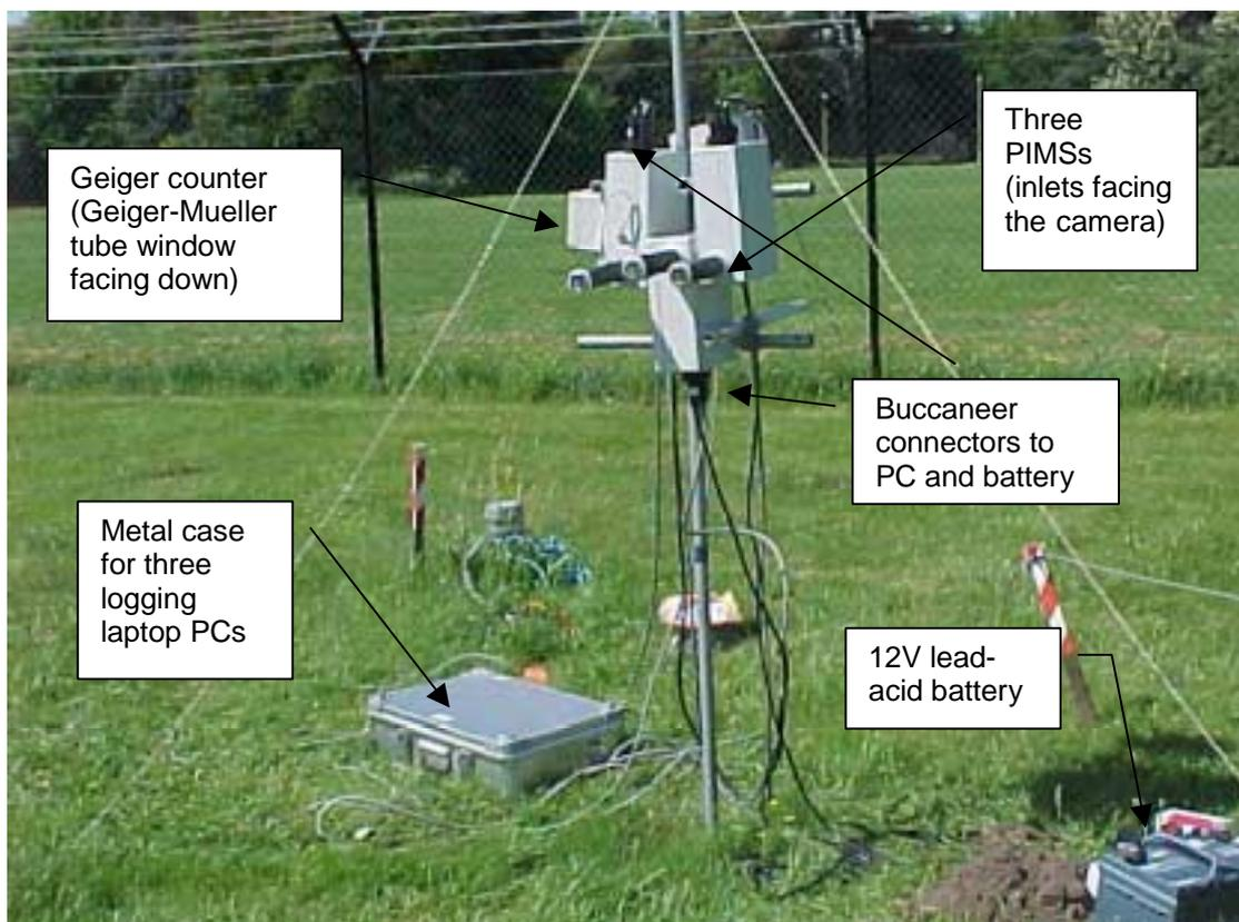
Figure 6.2 Photograph of the PIMs running at Reading University Meteorology Field Site.
