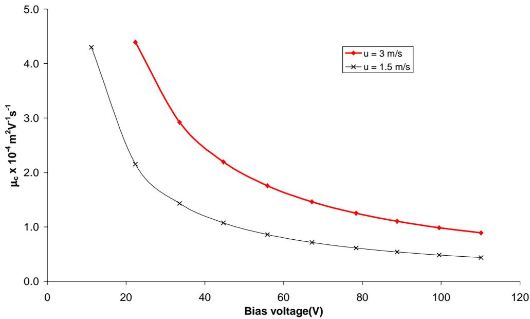
Figure 3.3 Critical mobility  $\mu_c$  against bias voltage at two flow rates for  $k = 0.00178 \text{ m}$ , the value used in the Gerdien experiments discussed in this chapter.
