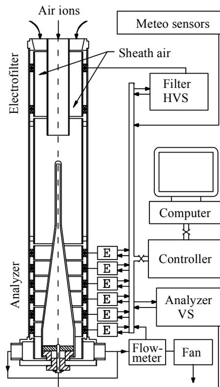
Figure 2.9 The Estonian small air ion spectrometer, from Hõrrak et al (2000). E is an electrometer, HVS high voltage supply, and VS voltage supply. The height of the spectrometer is 69.5 cm, and the diameter is 12.2 cm.
