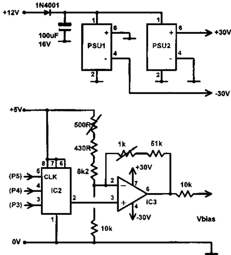
Figure 5.3 Schematic diagram of the bias voltage generator (from Aplin and Harrison, 2000). PSU 1 and 2 are transformer-isolated 30 V modules (type NMA12155) supplying non-inverting amplifier IC3 (OPA 445). A trimmable voltage offset is applied to IC3 to allow the unipolar generation of the IC2 (MAX 550A) to generate bipolar bias voltages.
