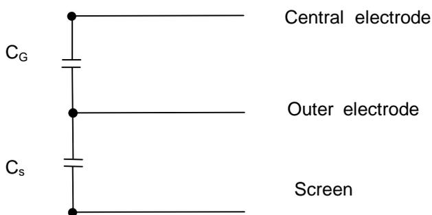
Figure 5.15 Schematic of the capacitances between the Gerdien condenser electrodes and screen.
