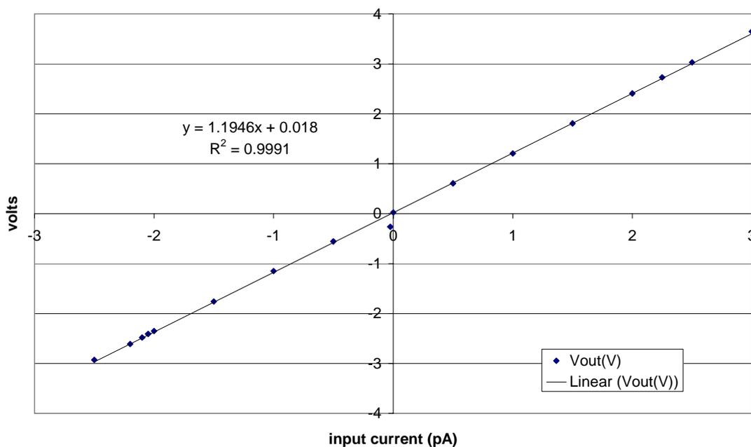
Figure 3.12 Resistive current amplifier calibration. The input current was generated using a series 1 T $\Omega$  calibration resistor ( $\pm 10\%$ ) driven using a dc millivolt calibrator ( $\pm 0.02\%$ ). The output voltage was measured using the Keithley 2000 digital voltmeter ( $\pm 35$  ppm).
