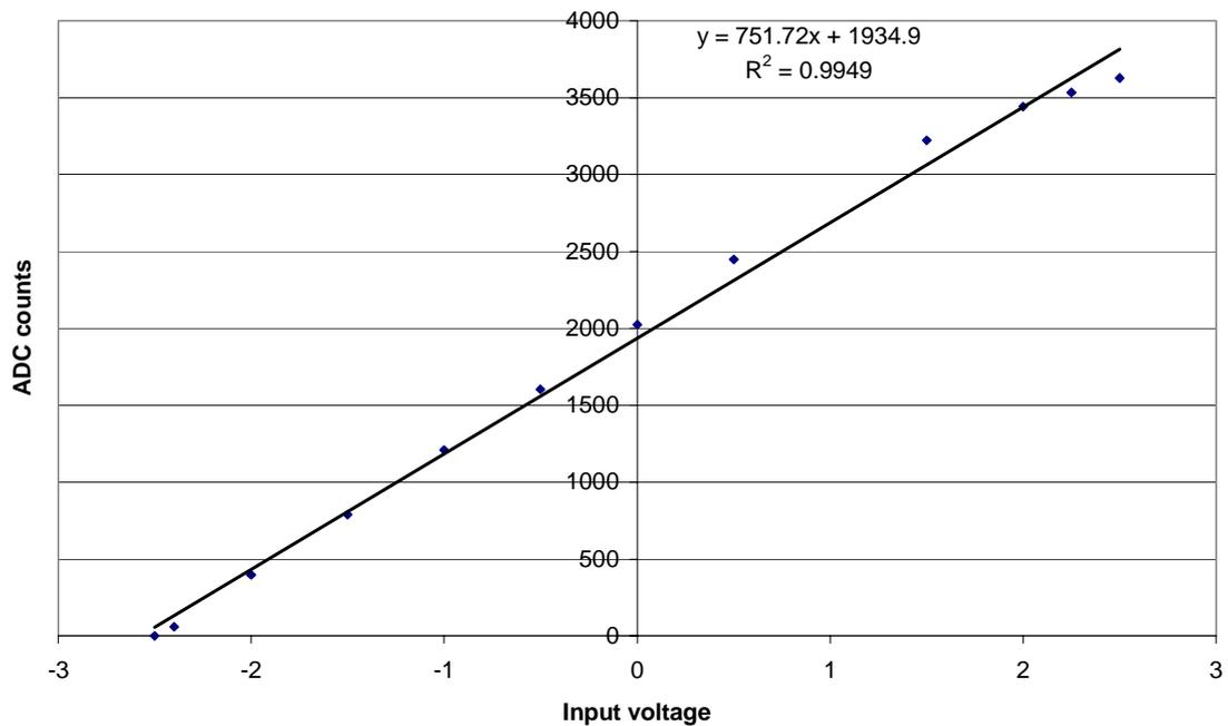
Figure 4.3 ADC calibration, with bipolar voltages from a millivolt calibrator. The linear response range is shown here.
