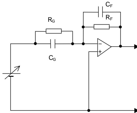
Figure 3.13 The Gerdien system's analogous electrical circuit. The Gerdien is a capacitor  $C_G \sim 8\text{pF}$ , and  $R_G$  is effectively the resistance of air (of order  $1\text{P}\Omega$ ). The op-amp and feedback resistor  $R_F$  ( $1\text{T}\Omega$ ) are the current amplifier.  $C_F$  is parasitic capacitance  $\sim 1\text{pF}$ . The cell was a millivolt calibrator, and provides a bias voltage from  $\pm 0\text{-}10\text{ V}$ .
