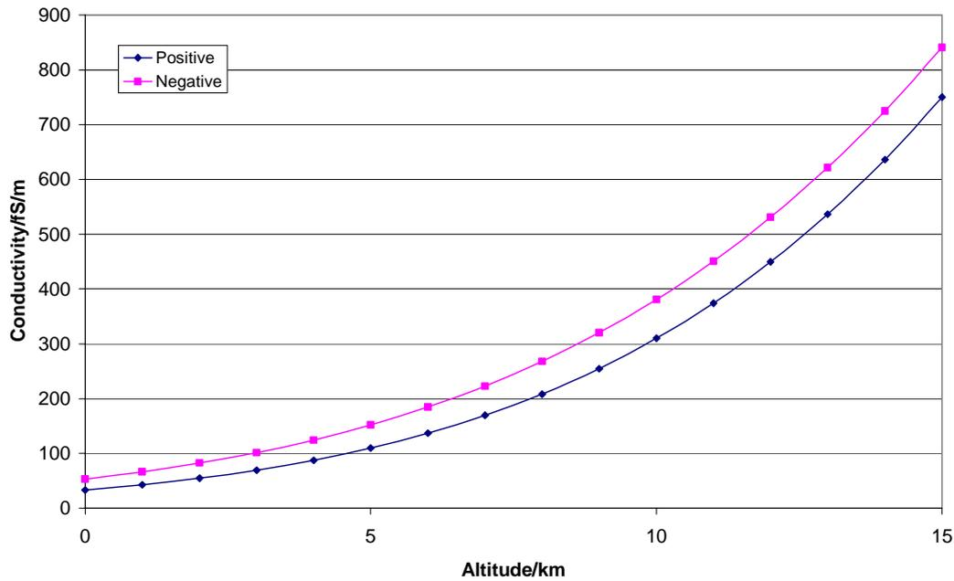
Figure 2.5 Variation of conductivity with altitude from Eq. 2.21 and Eq. 2.22, derived by Woessner *et al* (1958).
