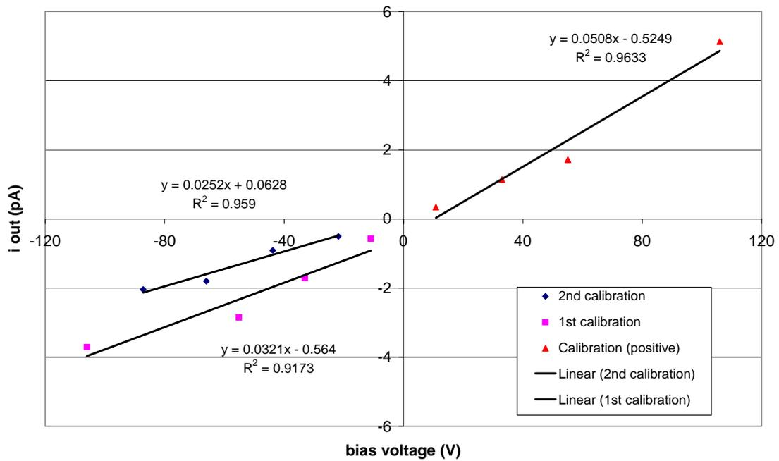
Figure 6.14 Ohmic response of Arizona Gerdien. The two tests at negative voltages were made approximately an hour apart.
