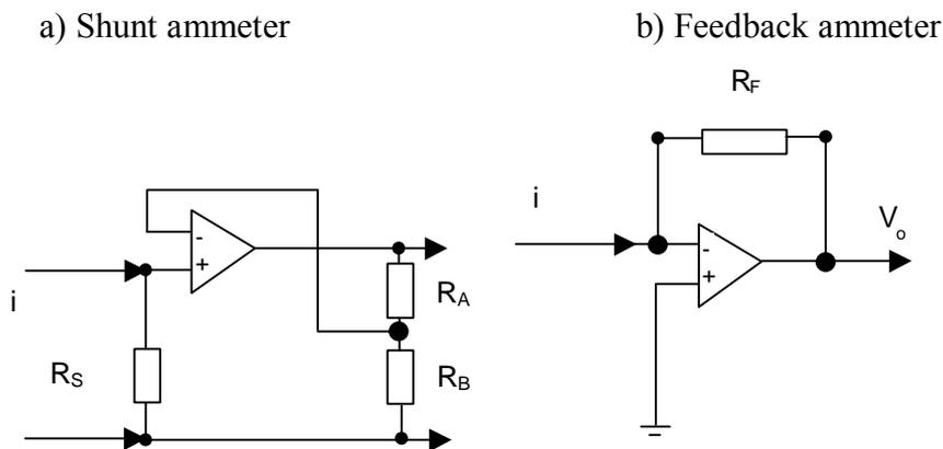
*Figure 3.4 Ammeters using op-amps, after Keithley (1992).  $R_F$  and  $R_S$  are the large value resistors.  $i$  is input current,  $V_o$  is output. Note that for the shunt ammeter (a), the signal joins the non-inverting input, and for the feedback ammeter (b), the inverting input.*
