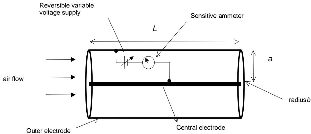
Figure 2.2 Schematic of a Gerdien condenser
