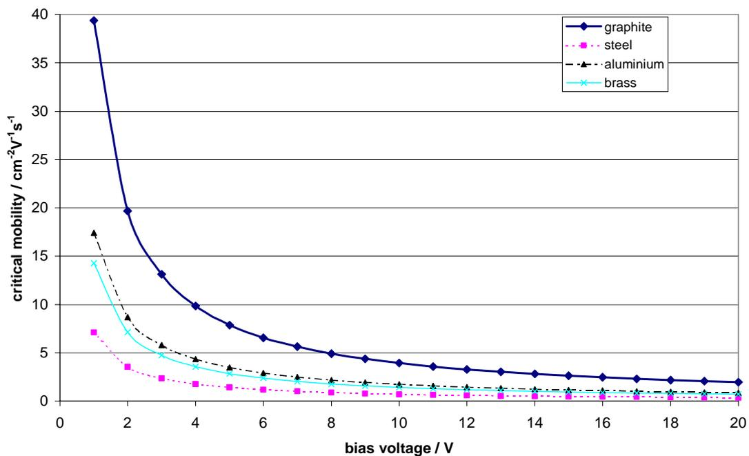
Figure 3.15 Variation of critical mobility ( $cm^2s^{-1}V^{-1}$ ) with voltage (V) for the four different tubes tested.
