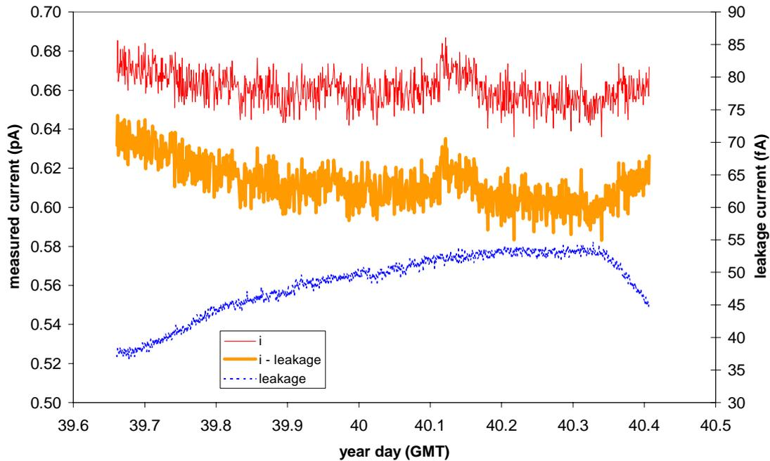
Figure 5.14 Comparison of measured  $i_m$  (thin trace), leakage  $i_L$  (thick trace) and  $(i_m - i_L)$  currents sampled every minute for 18 hours in the laboratory, in response to a resistively generated current of  $\sim 600$  fA.  $i_L$  is shown in the blue (dotted) trace on the right-hand axis.
