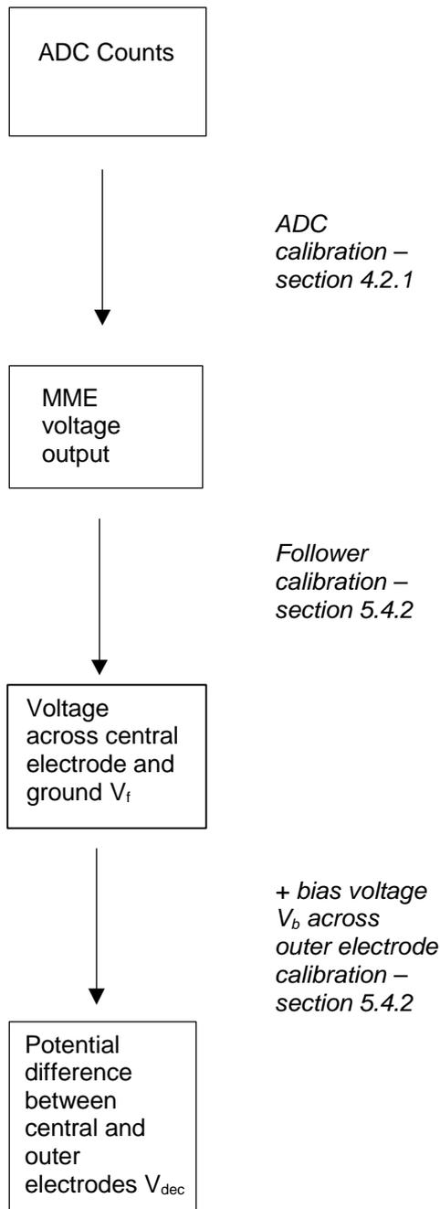
Figure 6.5 Schematic diagram showing the calibrations used to convert ADC counts stored by the logging PC, to the total potential difference across the outer and central electrodes.
