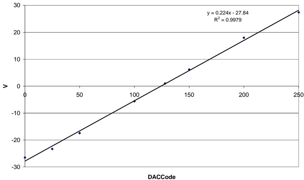
Figure 5.4 Bias voltage generator calibration, programming the DAC with the microcontroller and measuring the output voltage. Using a least squares linear fit to this data results in an error in the output voltage of  $\pm 2$  %, from the standard errors in the fit.
