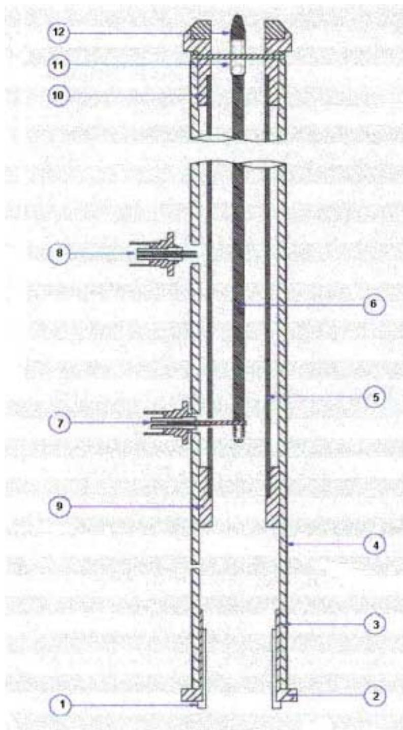
Figure 5.1 The principal components of the PIMS Gerdien. 1 indicates the fan position, 2 fan housing, 3 acrylic outer screen, 4 electrical outer screen (conductive tape), 5 outer electrode, 6 central electrode, 7 central electrode BNC connector, 8 outer electrode BNC connector, 9 outer electrode rear support, 10 outer electrode front support, 11 central electrode insulator, 12 inlet bullet-shaped cap.
