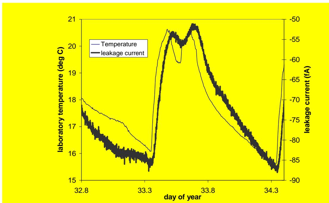
Figure 5.13 Diurnal cycle of laboratory temperature measured with a platinum resistance thermometer (Harrison and Pedder, 2000) and MME leakage current, found using modes 3 and 4, which is plotted on the right hand axis.
