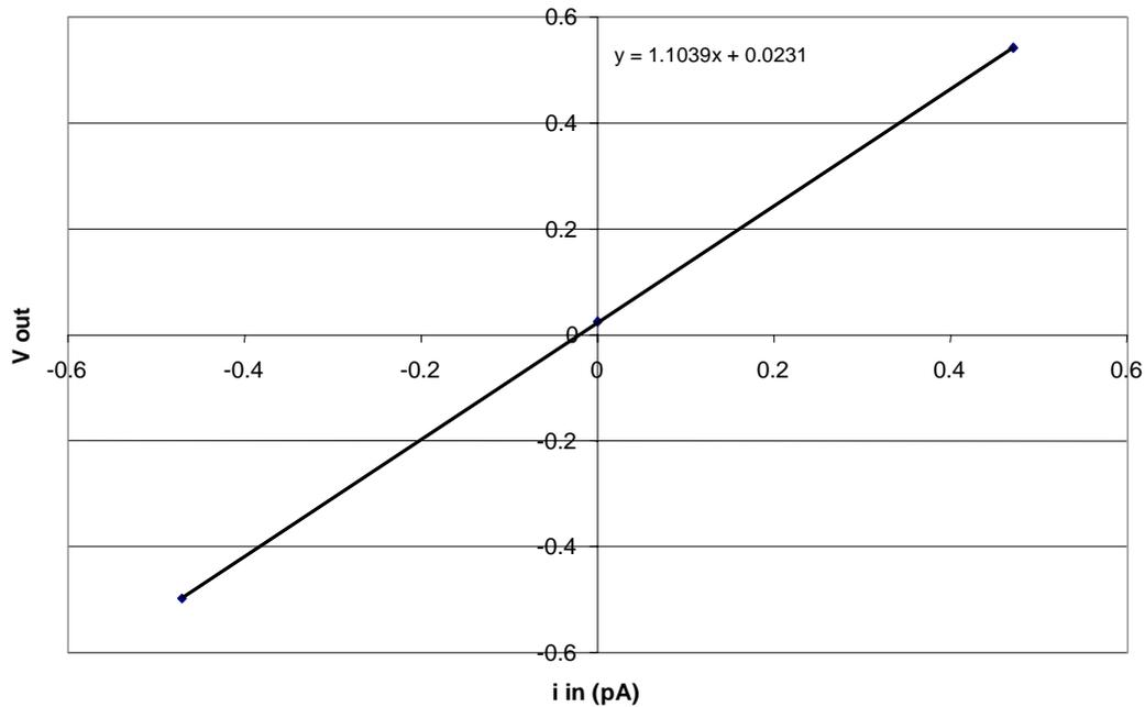
Figure 5.11 MME calibration in picoammeter mode, with currents generated from the precision voltage ramp connected to a 10 pF capacitor. The offset was measured when the picoammeter input was connected to the screened 10 pF capacitor, with the ramp generator disconnected. The picoammeter gain is  $(1.104 \pm 0.004)$  V/pA, and the offset is  $(2.3 \pm 0.1)$  mV (errors are the standard error in the least squares linear fit).
