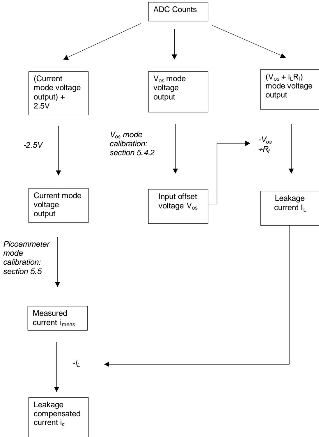
Figure 6.4 Schematic showing the calibration and correction procedures required to obtain a compensated current measurement. The three modes operate sequentially, for 10 s each. This procedure is repeated for measurements at each bias voltage.
