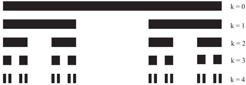
Fig. 1. Grids constructed following the first five orders of growth for the triadic Cantor fractal ( n = 2 and r = 1/3 ).
