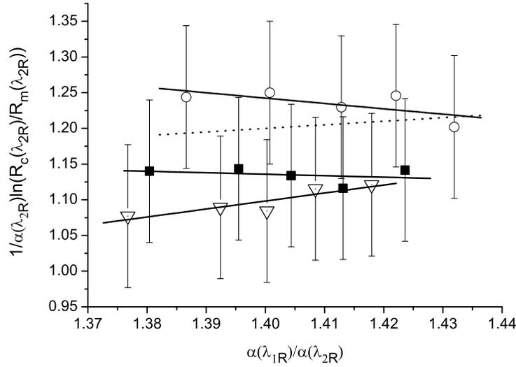
Fig. 10. Plot to determine  $d_1$  and  $d_2$ , as described in the text. Three solutions of different concentrations were measured: 0.001% (open circles), 0.0025% (filled squares) and 0.005% (open triangles). The dotted line indicates the predicted trend, calculated from the known system geometry. Errors were calculated according to equation 11 as described in the text.
