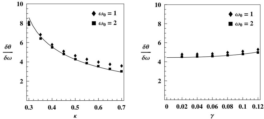
FIG. 2: The slope  $\frac{\delta\theta}{\delta\omega}$  in the Winfree model. On the left:  $\frac{\delta\theta}{\delta\omega}$  as a function of  $\kappa$  for two values of  $\omega_0$  and  $\gamma = 0.1$ . On the right:  $\frac{\delta\theta}{\delta\omega}$  as a function of  $\gamma$  for two values of  $\omega_0$  and  $\kappa = 0.45$ . The curves are independent of  $\omega_0$ .
