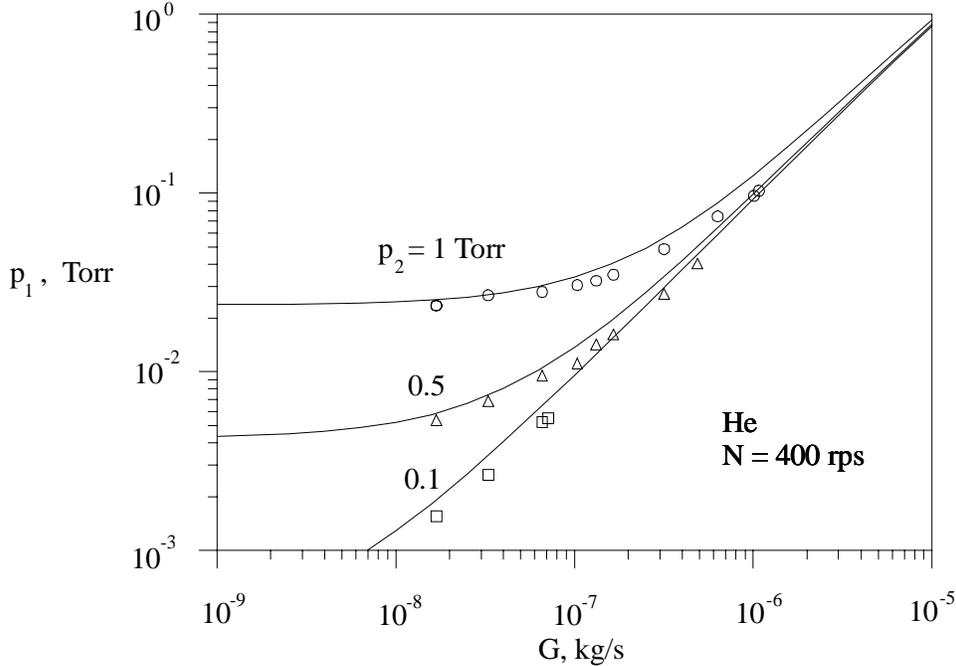
**FIGURE 1.** Inlet pressure versus gas flow rate at several outlet pressures.
