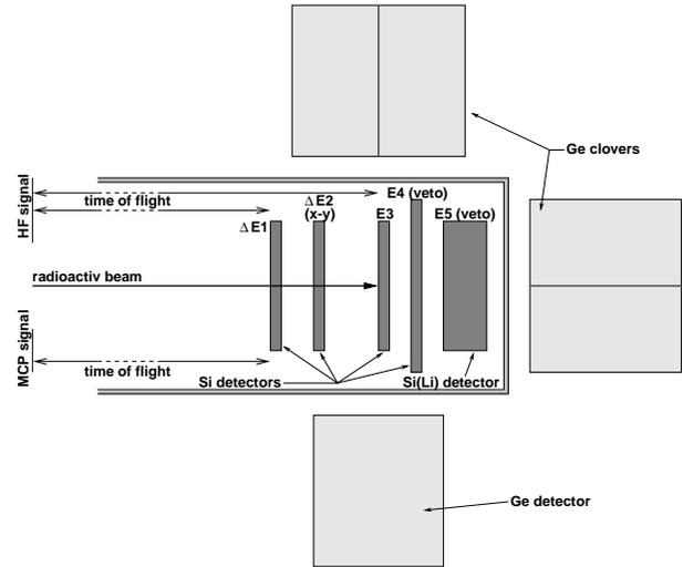
**Fig. 1.** Detection setup: Ions are implanted in the  $E3$  detector. The identification of isotopes is performed with the  $\Delta E1$  and  $\Delta E2$  energy loss information, several time-of-flight measurements, the total energy and position measurements. For details see ref. [2].
