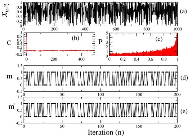
FIG. 3: (a) The transmitted signal including the message  $m$  at  $\alpha = 0.7$ ,  $\Lambda = 100$ , and  $\epsilon = 10^{-8}$ ; (b) The autocorrelation of the transmitted signal, which shows  $\delta$  function shape; (c) The probability distribution function of the transmitted signal  $x_{n-\tau}$ ; (d) The original message at transmitter side; (e) The decoded message at receiver side.
