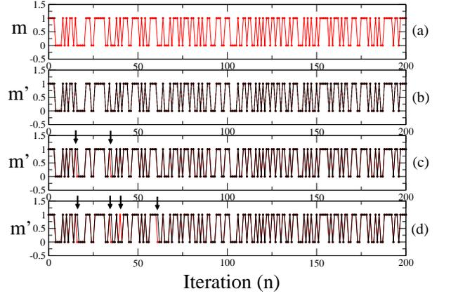
FIG. 4: The decoded messages for different values of the threshold  $\epsilon$  in the presence of noise of  $\max(\xi_n) = 10^{-6}$ . (a) The original message; (b) The decoded message with  $\epsilon = 2.5 \times 10^{-5}$ . (c) With  $\epsilon = 2.0 \times 10^{-5}$ ; (d) With  $\epsilon = 1.5 \times 10^{-5}$ . The arrows in (c) and (d) indicate the bit-flipped events in the decoded message
