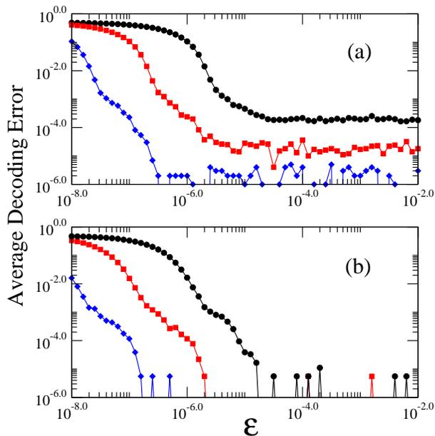
FIG. 5: The average decoding errors for different noise amplitudes as a function of the threshold  $\epsilon$ , where the points below  $10^{-6.0}$  are zero. Each datum point is the result of  $10^6$  bit transfer. Circles:  $\max(\xi) = 10^{-6}$ ; Squares:  $\max(\xi) = 10^{-7}$ ; Diamonds:  $\max(\xi) = 10^{-8}$ . (a) Without the error correction; (b) With the error correction. See Ref. [18] for details of the error correction method.
