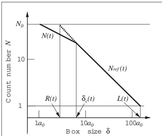
FIG. 2: Relation of  $\delta_c(t)$ ,  $N(t)$  and  $R(t)$  in the graph of log-log scale for the box size  $\delta$  and count number  $N$ . Cross-over effect and the maximum fluctuation are shown.
