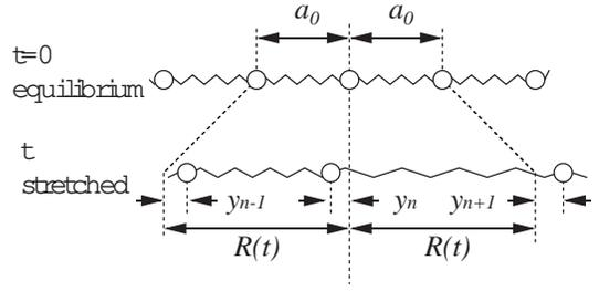
FIG. 1: Sketch of the extended chain used. At equilibrium, random and small fluctuations are assumed.
