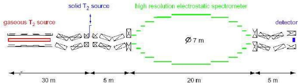
Fig. 16. Conceptual design for the KATRIN experiment for higher-precision measurements of the neutrino mass using the endpoint of the tritium  $\beta$ -decay spectrum.
