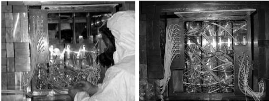
Fig. 8. Left picture: during the LIBRA detectors installation in HP Nitrogen atmosphere. Right picture: view at end of the detectors installation. All the used materials have been deeply selected for radiopurity (see for example the cables with teflon envelop).
