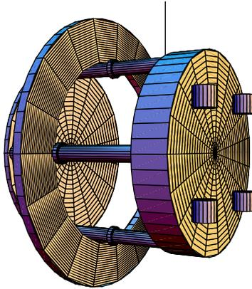
Figure 2: Rendition of the ISLV pendulum. The pendulum is made of fused silica parts with a total mass of 240g. The diameter is roughly 8cm. Four moveable trim masses are visible on surface of the thick disk.
