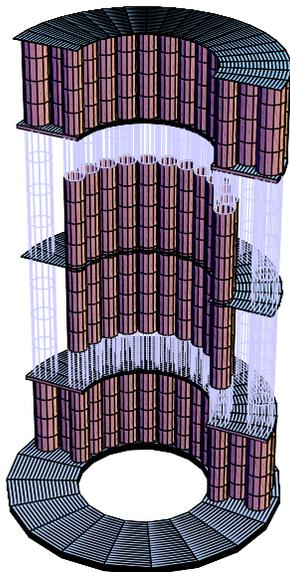
Figure 3: Rendition of the ISLV source mass. The mass is composed of several hundred precision machined solid stainless steel cylinders. The wireframe components are hollow steel tubes. The diameter of the base is approximately 1m.
