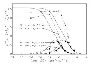
FIG. 2. Relaxation rates of free induction decay  $(1/T_2^*, \text{GE})$  and spin echo experiments  $(1/T_2, \text{ echo time} = 50 \text{ ms}, \text{SE})$ . Simulation (sim.) and theoretical (solid lines)results are compared for a capillary radius of  $2.5\mu\text{m}$  and  $7.5\mu\text{m}$ . Other parameters are as in Fig. 1.
