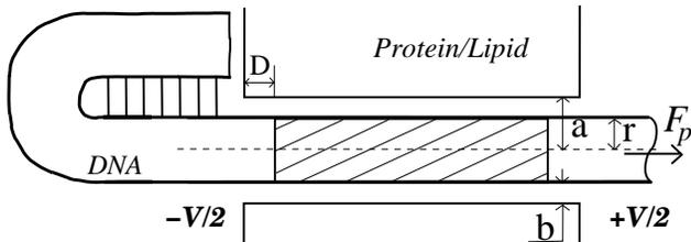
FIG. 3: Unzipping of the DNA hairpin with the help of the voltage induced pulling force  $F_p$  results in DNA translocation through the channel to the right. Alternatively DNA can escape against electric field to the left. The hairpin is shown schematically with the bound base pairs presented by short straight lines. There are  $M$  base pairs in the hairpin,  $N_0$  bases in the channel and  $K$  bases in the tail to the right of the channel.
