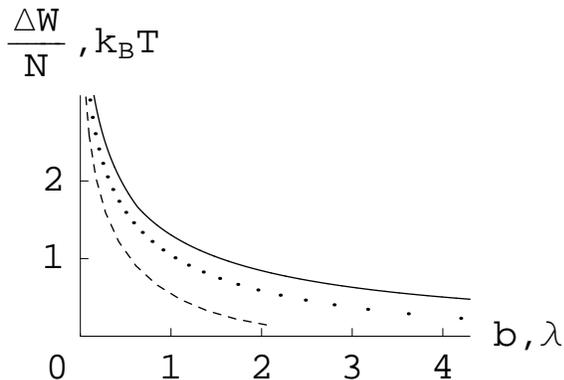
FIG. 9: Free energy of the capture barrier per one screened DNA charge in the channel as a function of  $b$  (in units of  $\lambda$ ) for  $c = 0$  (solid line),  $ce^2/(l_B \sigma^2) = 0.1$  (dotted line) and  $ce^2/(l_B \sigma^2) = 1$  (dashed line).
