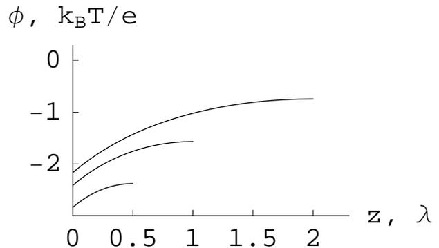
FIG. 8: The potential  $\phi$  as a function of  $z$  for  $b/\lambda = 0.5, 1$  and  $2$  (from bottom to top), at ion concentration  $ce^2/(l_B\sigma^2) = 1$ . Here the Gouy-Chapman length  $\lambda = k_B T \kappa / (2\pi\sigma e)$  is the unit of distance.
