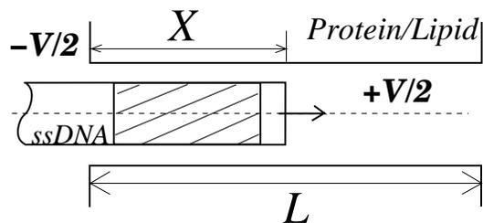
FIG. 2: The side view of a ssDNA molecule entering the channel.
