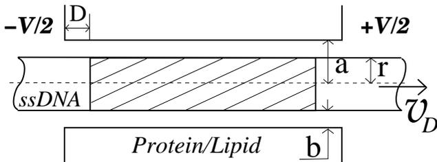
FIG. 1: The side view of the membrane and the channel with captured DNA. All DNA phosphates in the shaded part are neutralized by  $K^+$  ions. The contact layer on each end has the length  $D$ . The arrow shows the direction of DNA motion.
