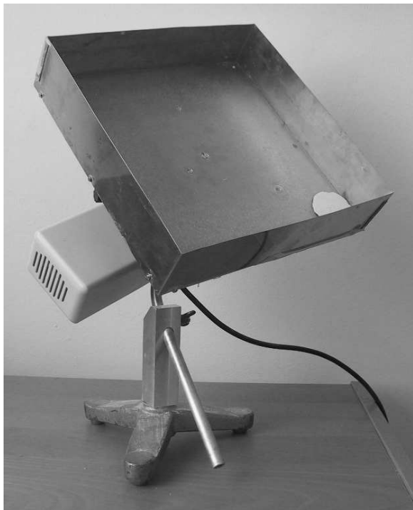
FIG. 2: The wearing apparatus used for the laboratory experiments. The rotating metal tray is 30 \times 30 \times 7 \text{ cm}^3 .
