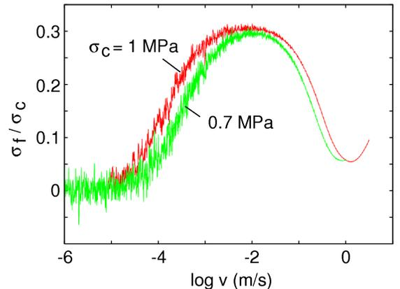
FIG. 10: The frictional shear stress  $\sigma_f$  as a function of the logarithm of the sliding velocity of the rubber block. For the temperature  $T = 20$  °C and for the (zero-temperature) depinning stresses  $\sigma_c = 1$  MPa and  $\sigma_c = 0.7$  MPa. All other parameters as in Fig. 5.
