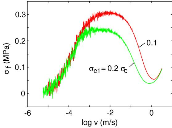
FIG. 8: The frictional shear stress  $\sigma_f$  as a function of the logarithm of the sliding velocity of the rubber block. For the temperature  $T = 20$  °C and for the critical stresses (below which steady sliding becomes metastable)  $\sigma_{c1} = 0.1\sigma_c = 0.1$  MPa and  $0.2$  MPa. All other parameters as in Fig. 5.
