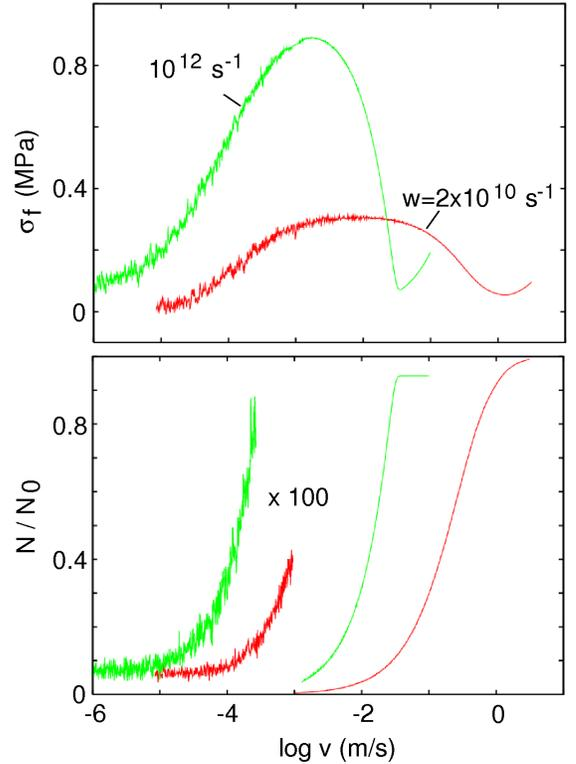
FIG. 9: The frictional shear stress  $\sigma_f$  as a function of the logarithm of the sliding velocity of the rubber block. For the temperature  $T = 20$  °C and for the probability rates per unit time to return to the pinned state (when  $\sigma < \sigma_{c1}$ )  $w = 2 \times 10^{10} \text{ s}^{-1}$  and  $w = 10^{12} \text{ s}^{-1}$ . All other parameters as in Fig. 5.
