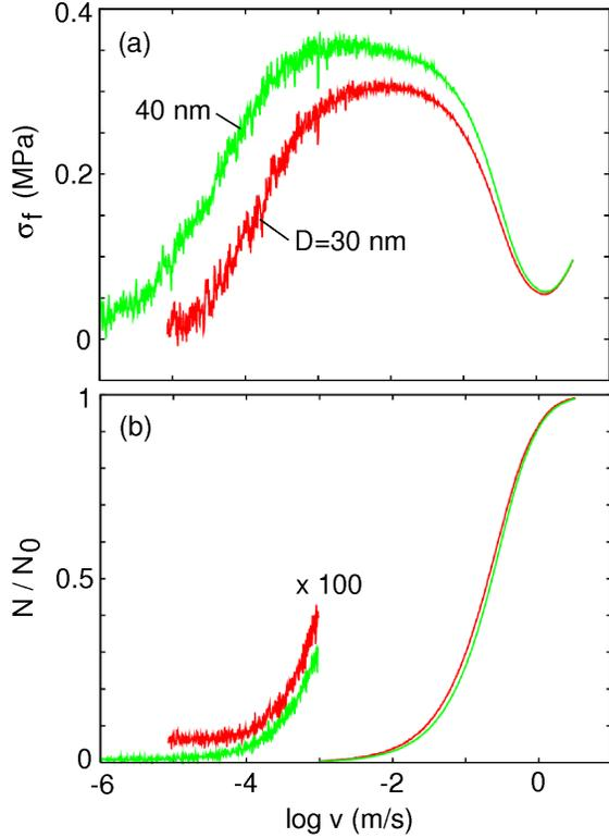
FIG. 6: The frictional shear stress  $\sigma_f$  as a function of the logarithm of the sliding velocity of the rubber block. For the temperature  $T = 20^\circ\text{C}$  and for the stress block sizes  $D = 30$  and  $40$  nm. All other parameters as in Fig. 5.
