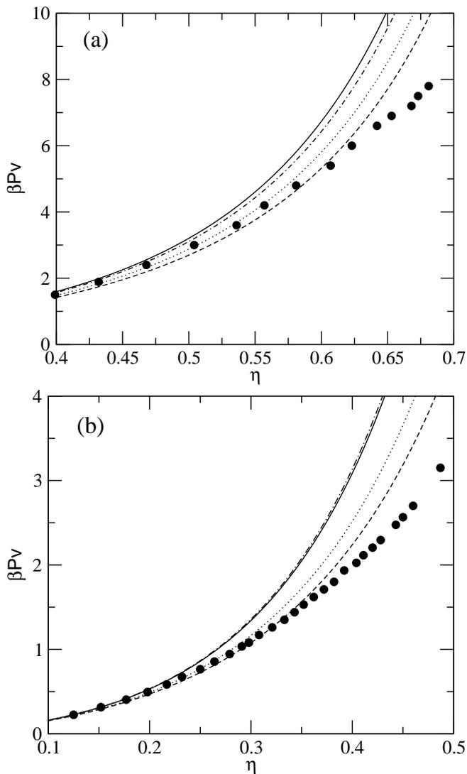
FIG. 4: Results from MC simulations (filled circles) on a system of 10800 HRs with  $\kappa = 3$  (a), and  $\kappa = 9$  (b). Dot-dashed line: Eq. (7) with  $B_3$  calculated from MC integration, dashed line: SPT, dotted line: Boublik proposal, and solid line: our proposal [The  $B_3$  from Eq. (2) with  $\{\alpha = 1.611, \beta = 0.514\}$ ].
