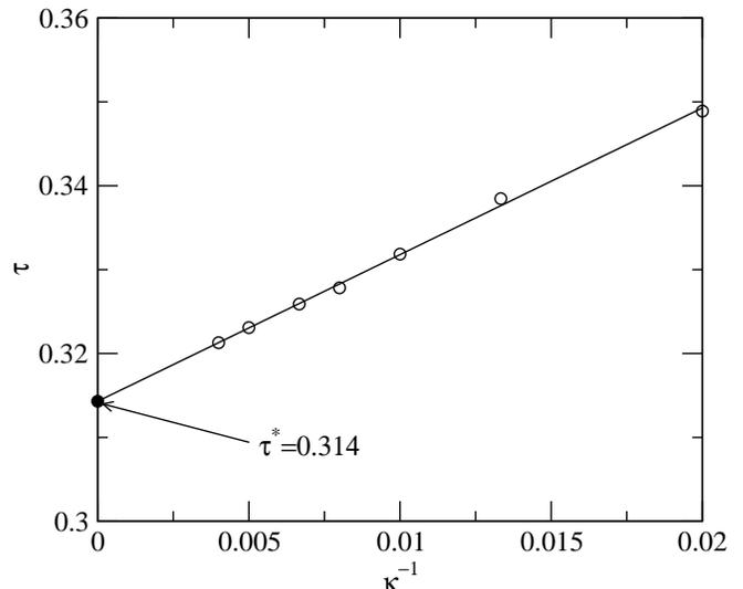
FIG. 8: The coefficient  $\tau(\kappa)$  [see Eq. (48)] as a function of  $\kappa$  for a discrete set of  $\kappa$ 's (open circles) calculated via Monte-Carlo integration. The straight line calculated from mean square approximation intersects the ordinate at the value indicated in the figure.
