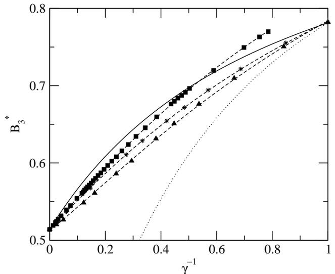
FIG. 2: Reduced virial coefficient  $B_3^*$  as a function of the anisometric parameter  $\gamma$ . Simulation results are shown for hard rectangles (squares), discorightangles (asterisk), and ellipses (triangles). The solid and dotted lines are the results from Eq. (13) with  $(\alpha, \beta) = (1.611, 0.514)$ , and  $(\alpha, \beta) = (2, 1/8)$  respectively. Also are shown with dashed lines the best fits from Eq. (22).
