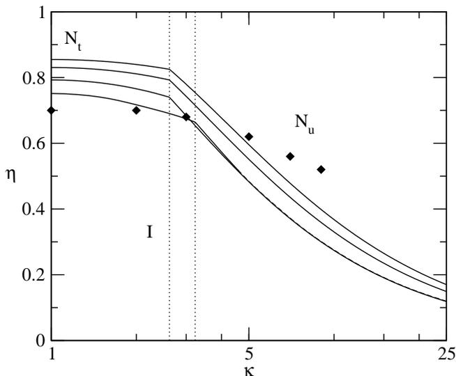
FIG. 12: Spinodals of the transitions between the isotropic and orientational ordered phases. From top to bottom are shown the results from the SPT, the EOS with the approximated  $b_3$  (the Boublík, and our proposal), and from the EOS with the exact  $b_3$ . The dotted lines represent the position of the tricritical points common to all the approximations and that corresponding to the exact  $B_3$ . Also are shown the simulation results.
