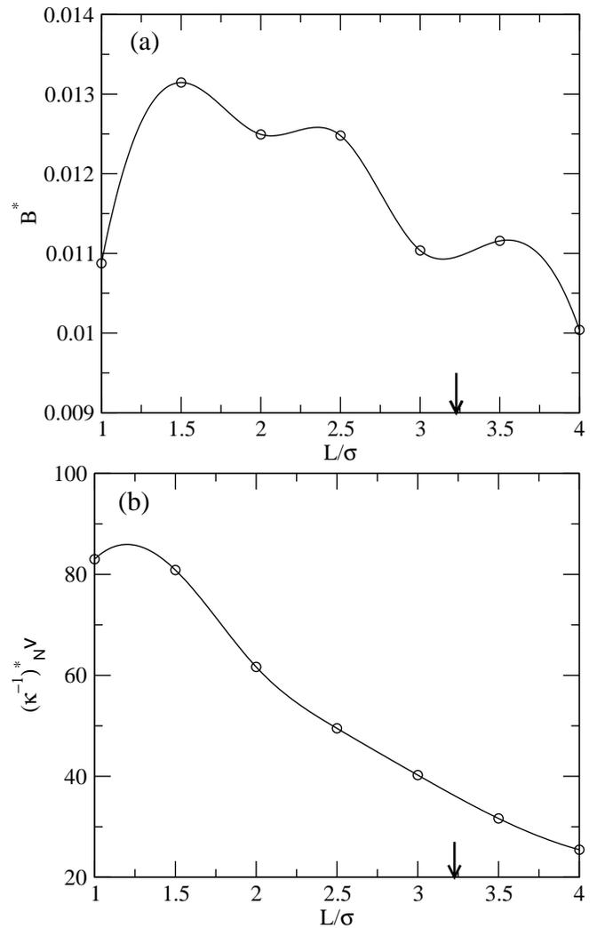
FIG. 6: The coefficient  $B^*$  (a), and the inverse of the compressibility factor  $(\kappa_N^{-1}v)^*$  (b) at the  $I-N_t$  bifurcation point as a function of the aspect ratio calculated for a discrete set of values (open circles). Both magnitudes are always greater than zero, so the  $I-N_t$  is always of second order. The arrow indicates the maximum aspect ratio of  $N_t$  phase stability.
