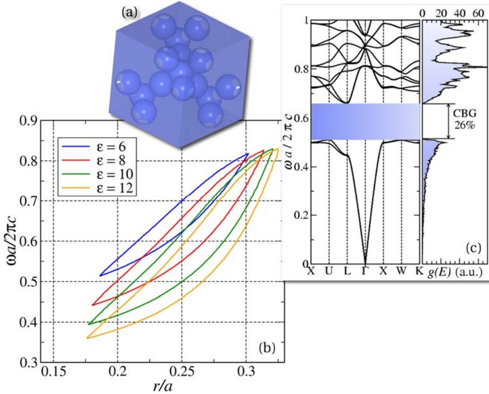
Fig. 5. Band gap map at selected values of  $\epsilon$  for the pyrochlore lattice of air spheres in dielectric. (a) Pictorial representation of the lattice at  $r/a = 0.27$  (radius of the air sphere at which the maximum PBG is attained for  $\epsilon = 12$ ). (b) Band gap map for this structure. (c) Band structure and density of states at  $r/a = 0.27$  for  $\epsilon = 12$ . See the caption of Fig. 4 for the computational details.
