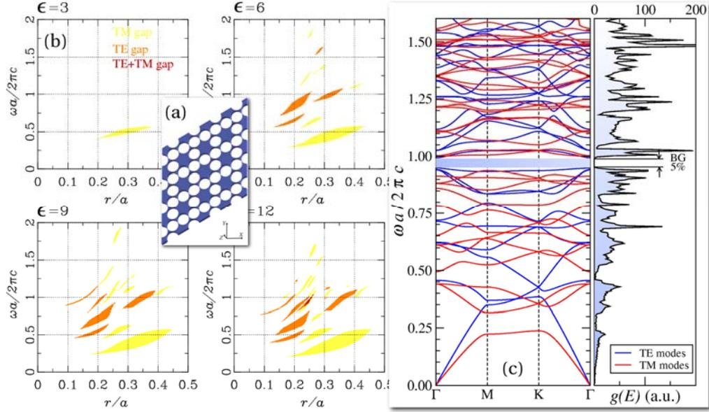
Fig. 3. Band gap map at selected values of  $\epsilon$  for the kagomé lattice of air rods in dielectric. (a) Pictorial representation of the lattice at  $r/a = 0.24$  (radius of the air cylinders at which the maximum BG is attained for  $\epsilon = 12$ ). (b) Band gap map for this structure. (c) Band structure and density of states at  $r/a = 0.24$  for  $\epsilon = 12$ ; the blue stripe delimits the photonic band gap. See the caption of Fig. 2 for the computational details.
