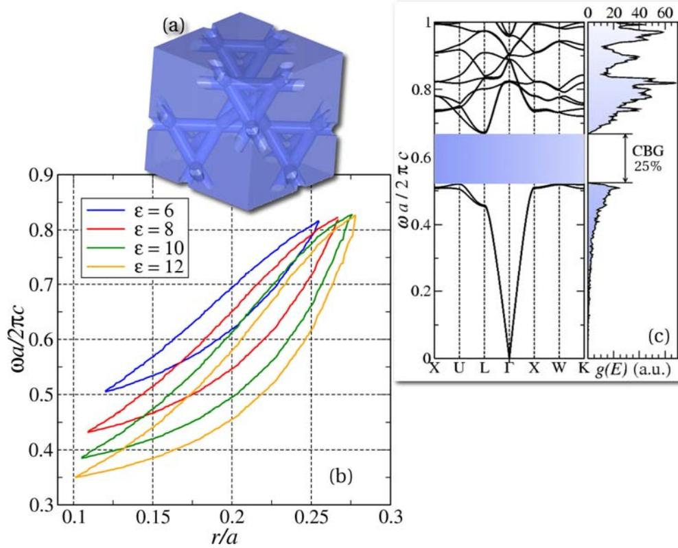
Fig. 6. Band gap map at selected values of  $\epsilon$  for the pyrochlore lattice of air rods in dielectric. (a) Pictorial representation of the lattice at  $r/a = 0.10$ . (b) Band gap map for this structure. (c) Band structure and density of states at  $r/a = 0.24$  for  $\epsilon = 12$ ; the gray stripes delimit the photonic band gap. See the caption of Fig. 4 for the computational details.
