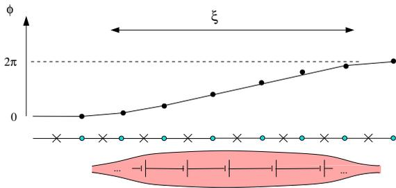
FIG. 10: Schematic of a QPS in a continuous wire. The size of the core of a QPS — in which the superconductivity is suppressed — is of order the superconducting coherence length  $\xi$ . The wire can be considered as the limit of a chain of grains whose separation,  $a$ , is much smaller than  $\xi$ .
