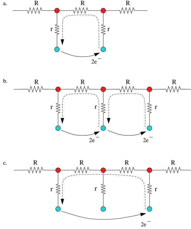
FIG. 8: (a) Cooper pair tunneling event, between two neighboring grains (solid line): the basic process for weak Josephson coupling. Charge relaxation is via the resistance  $2r + R$  (dotted line). (b) Two nearly simultaneous pair-tunnels involving a common grain: the current through the conversion resistance  $r$  of that grain cancels giving rise to an effective interaction between the two pair-tunnels. These two pair tunnels can renormalize into a pair-tunnel over two junctions (c).
