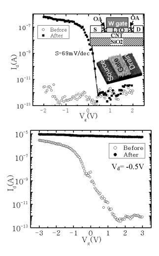
FIG. 3: (a) Transfer characteristics of a W-top-gated CNT-FET before and after **OA** "extension doping" at  $V_{ds} = -0.5$ V. S is 69 mV/dec post doping. The inset shows a schematics and a SEM picture of the device; (b) transfer characteristics of a bottom-gated CNTFET device before and after degenerate **OA** doping where a p-CNFET was transformed into an almost metallic tube.
