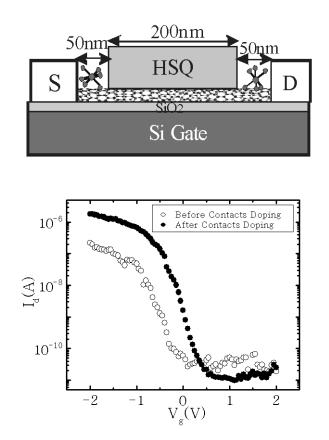
FIG. 2: (a) Cross-section schematics of a HSQ patterned CN-FET selectively doped by **OA** at the source-drain contacts; (b) transfer characteristics of the device before and after selective **OA** doping at  $V_{ds} = -0.5 V$ .
