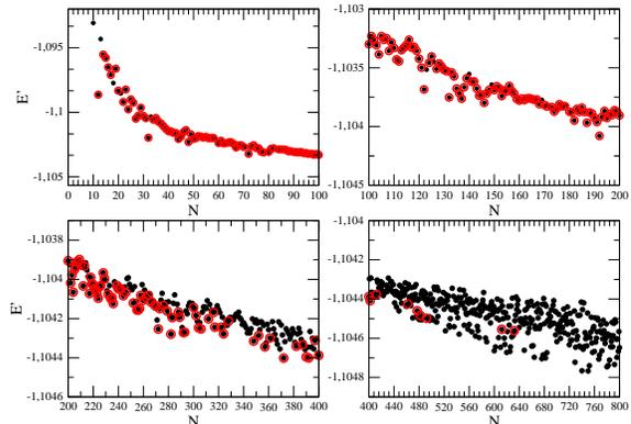
FIG. 2:  $E' = (2E - N^2)/N^{3/2}$  vs.  $N$ .  $E'$  is defined using Eq. (1). Energies are plotted with black dots and are encircled in red if the associated presumed global minimum energy configuration has no dislocation defects.
