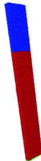
FIG. 1: (color online) A representative example of the flowing granular slab of height H = 300 . In this cohesive granular slab ( A = 0.8 ) the system separates into a solid-like plug (blue) sliding upon a flowing granular bed (red). The rough surface of inclined plane is shown in green.
