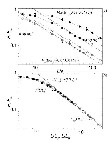
**Figure 6.** Average Fano factor F and its high-frequency counterpart  $F_{\infty}$  (Eqs. (26) and (27), respectively) as functions of conductor length L normalized to: (a) the localization length a, and (b) the scaling lengths  $L_c$  (for F) and  $L_h$  (for  $F_{\infty}$ ) (see Fig. 7 below), for two values of applied field at  $\chi = 0.5$ , T = 0 and  $W \gg L_c$ . Straight lines are the best fits to the data (using Eqs. (13) and (28)), while dashed curves are only guides for the eye.
