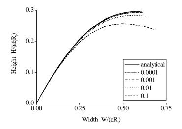
Figure 9: Deposit ring profile: dependence of the height of the phase boundary H on the width of the deposit ring W. The solid curve is the analytical result in the limit  $\chi_i/p \to 0$ ; the other curves are the numerical results. Different numerical curves correspond to different initial concentrations of the solute; values of parameter  $\chi_i/p$  are shown at each curve. The vertical scale is different from the horizontal scale by a factor of  $\theta_i \ll 1$ .
