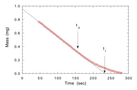
Figure 7: Mass of a drying drop as a function of time. Experimental results, after Refs. [23, 24]. The line running through the data is a linear fit. (Courtesy Robert Deegan.)
