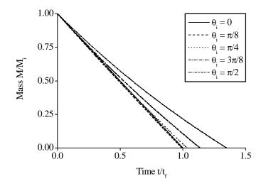
Figure 14: Numerical results: dependence of water mass M on time t. Different curves correspond to different initial contact angles; values of parameter  $\theta_i$  are shown at each curve. The analytical result [Eq. (66)] in limit  $\theta_i \to 0$  is also provided (the solid curve).
