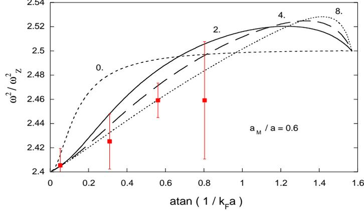
FIG. 2. Reduced axial mode frequency squared as a function of  $\arctan(1/k_F a)$  for the model Eq. 4 with the value of  $a_M/a = 0.6$  of Petrov *et al* and for  $c = 0, 2, 4$  and  $8$ . The filled squares, with error bars, are the data of Bartenstein *et al*.
