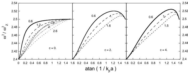
FIG. 1. Reduced axial mode frequency squared as a function of  $\arctan(1/k_F a)$  for the model Eq. 4 for  $c = 0, 2$  and  $4$ , and values of  $a_M/a$  as indicated near the various curves. For comparison we have also plotted with the  $c = 0$  case, as the thin line, the result of the model of Ref.13  $f(y) = 1/2 - (1/\pi) \arctan(\pi y/2)$ .
