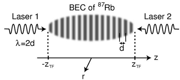
Fig. 1. BEC of Rb atoms is confined along the  $z$  and  $r$  directions by harmonic traps with frequencies  $\nu_z$  and  $\nu_r$  respectively. The condensate consists of  $5 \times 10^4$  atoms of  $^{87}\text{Rb}$ . Counter-propagating laser beams of wavelength  $\lambda$  form a potential of period  $d = \lambda/2$ .
