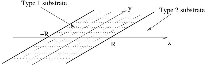
Figure 1: A schematic illustration of a planar substrate containing a stripe-like inhomogeneity. The wetting temperature of the stripe ( $T_{W1}$ ) is assumed lower than the substrate 2 wetting temperature ( $T_{W2}$ ). The domain width ( $2R$ ) is considered much larger than bulk correlation lengths.
