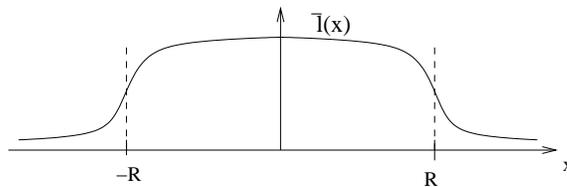
Figure 2: Schematic plot of the  $y = \text{const}$  section of the fluid density in the vicinity of the stripe, and the corresponding equilibrium shape of the liquid-vapor interfacial profile denoted by  $\bar{l}(x)$ .
