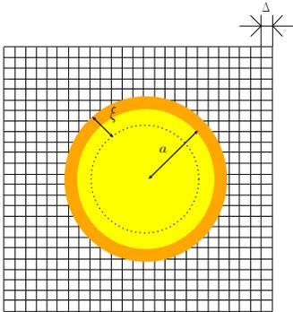
FIG. 2: Schematic representation of the cross section of geometry around the rod.  $\Delta$  is the lattice spacing,  $a$  is the rod radius, and  $\xi$  is the interfacial thickness. The rod surface now has a finite volume  $\sim 2\pi a\xi$  supported by several grid points on the fixed Cartesian coordinate.
