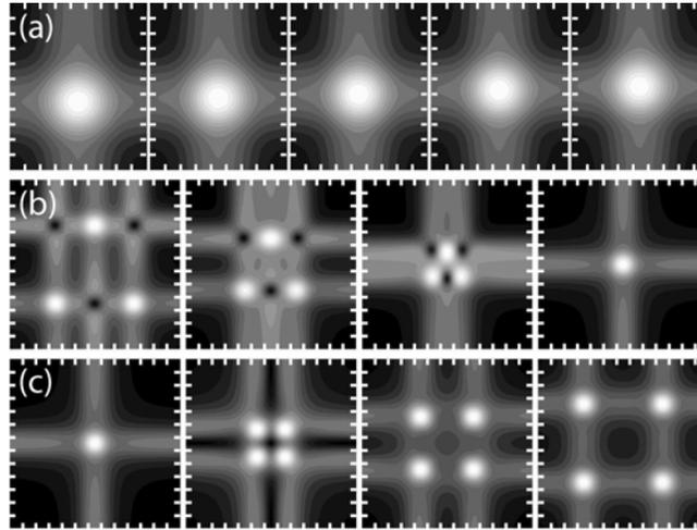
FIG. 2. Computed patterns of the magnitude of the magnetic field on the top surface of a matrix that demonstrate its principle of operation. The white ticks indicate wire positions and the total thickness of the two insulating layers is equal to the wire pitch. To produce a given magnetic pattern, the current in every wire was optimized using least-square fits.
