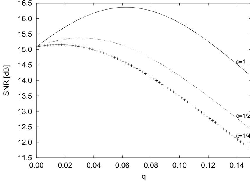
Fig. 2. Signal-to-noise ratio (SNR) for the linear transmitter (24) with various correlations between the noises:  $c = 1$  (solid line),  $c = 1/2$  (broken line),  $c = 1/4$  (crosses). Amplitude of the signal  $A = 1$ , frequency  $\Omega = 2\pi$ . Other parameters as on Fig. 1. Curves with  $c' = -c$  and  $b' = -b$  are identical to those presented above, cf. Eq. (18).
