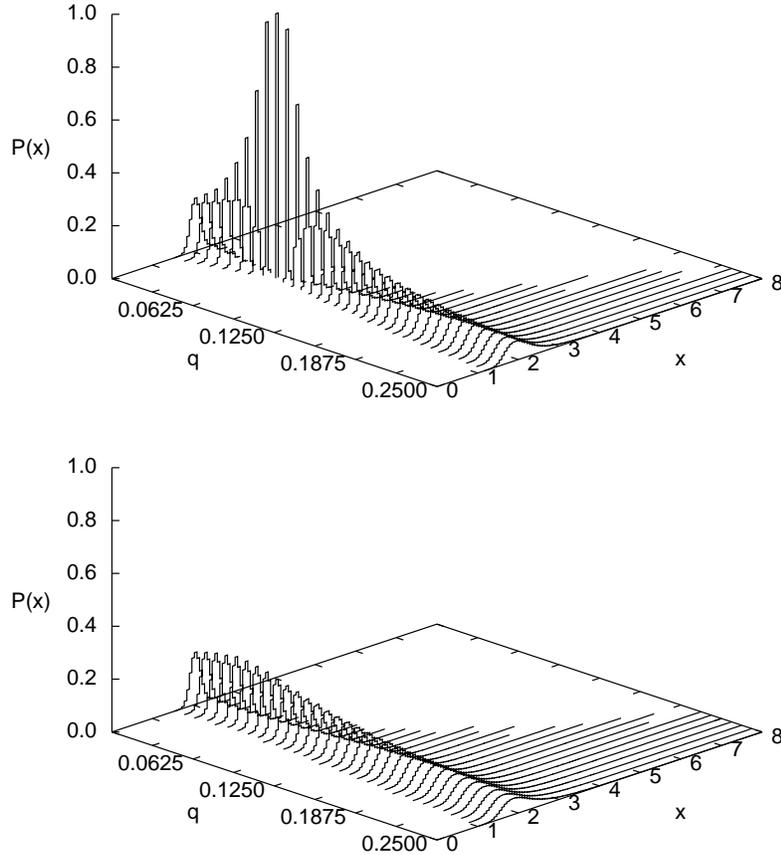
Fig. 1. Average distributions of values of  $x(t)$  described by Eq. (23) as a function of the additive noise level,  $q$ . Parameters are:  $a = 2$ ,  $b = 1$ ,  $p = 0.125$ . The correlations are  $c = 1$  (upper panel) and  $c = 0.5$  (lower panel).
