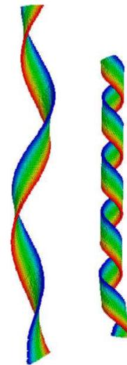
FIG. 4: (Color online) Two ribbons grown with the same elastic parameters, but with different orientations of the director representing the molecular tilt. In the left case, the tilt is aligned along the long axis of the ribbon, but in the right case it is aligned along the short axis. This change in the tilt direction reverses the handedness of the ribbon, and greatly changes the radius and pitch.
