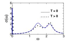
Figure 1.1. Schematic representation of the typical behavior of the conductivity for a clean metal.
