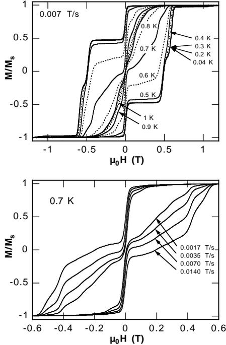
Fig. 1. Normalized magnetization versus applied magnetic field. The resulting hysteresis loops are shown at (a) different temperatures and (b) different field sweep rates. Note that the loops become temperature-independent below about 0.3 K but are still sweep-rate-dependent owing to resonant quantum tunnelling between discrete energy states of the  $\text{Mn}_4$  SMM.
