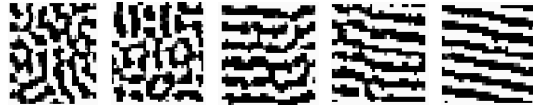
FIG. 7. Snapshots at C = 50 , \phi_H = 0 , and \chi N = 11.1, 11.2, 11.3, 11.4 , and 11.5 . White points: 0 < \bar{\phi}_A < 0.49 , gray points: 0.49 \leq \bar{\phi}_A < 0.51 , black points: 0.51 \leq \bar{\phi}_A \leq 1 . All runs were started from disordered configurations.
