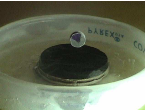
FIG. 1: Photograph of experimental setup. A YBCO disk rests on a metal base that is submerged in liquid N_2 . A Nd_2Fe_{14}B magnet levitates on top of the superconductor.
