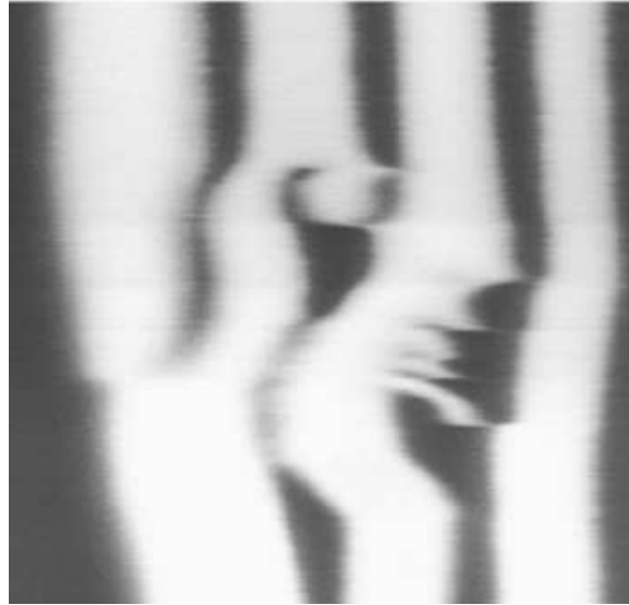
Fig. 5. Blowup of the center part of Figure 2 emphasizing a ‘turbulent’ event. Time goes down. The vertical axis corresponds to a total of 10 hours. A thin dark band is seen to nucleate and to perturb neighboring bands.
