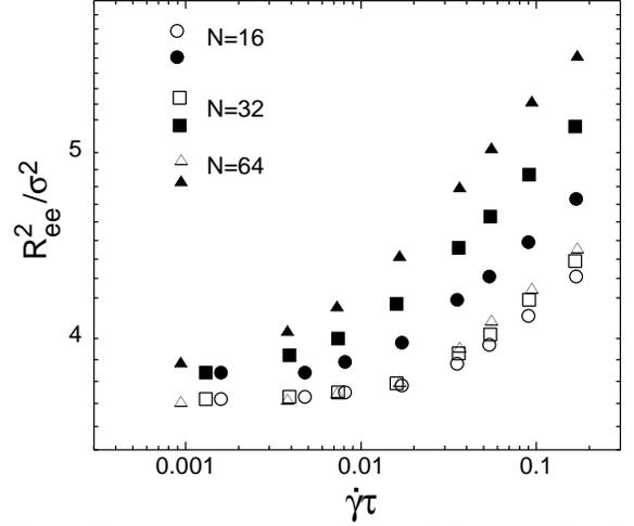
FIG. 8. The mean square end-to-end distance of 4 bead segments at the middle (filled symbols) and ends (open symbols) of polymers with the indicated  $N$  as a function of shear rate. The ends show the same behavior for all  $N$ . The middles begin to stretch at a lower shear rate that decreases with increasing  $N$ .
