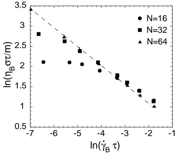
FIG. 3. Bulk viscosity  $\eta_B$  as a function of shear rate  $\dot{\gamma}_B$ , for polymers of length  $N = 16, 32$  and  $64$ . As  $N$  increases, shear thinning is observed at lower values of  $\dot{\gamma}_B$ . The dashed line shows a power law fit  $\eta_B \sim \dot{\gamma}^{-0.47}$ .
