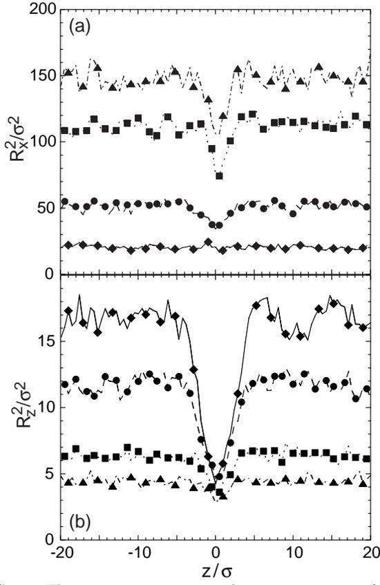
FIG. 6. The mean square  $x$  and  $z$  components of the end-to-end vector as a function of center of mass height for  $N = 32$  polymers at wall velocities  $v_w = 0.1\sigma/\tau$  (diamonds),  $0.5\sigma/\tau$  (circles),  $2\sigma/\tau$  (squares) and  $5\sigma/\tau$  (triangles). Corresponding bulk shear rates are given in Table I.
