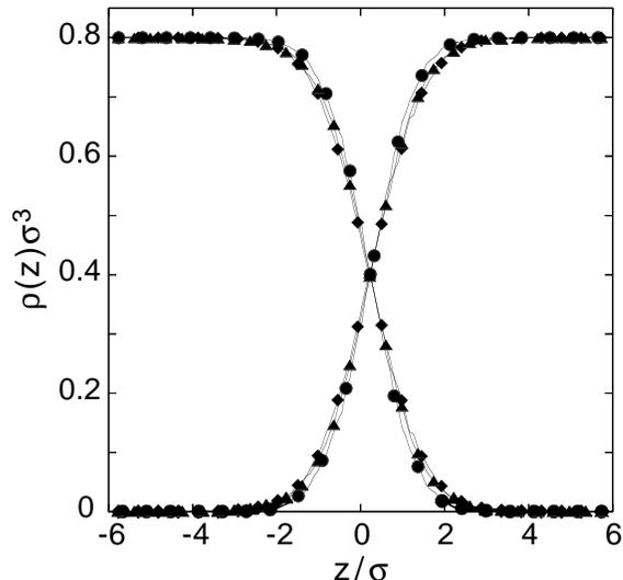
FIG. 1. Densities of type A (decreasing curves) and B (increasing curves) beads showing that the interface width is insensitive to chain length and shear rate. The immiscibility parameter is  $\epsilon^* = 3.2$  and circles are for  $N = 64$ ,  $v_W = 0.1$ ; diamonds are for  $N = 64$ ,  $v_W = 5.0$ ; and triangles are for  $N = 16$ ,  $v_W = 5.0$ . Corresponding values of  $\dot{\gamma}_B$  are given in Table I.
