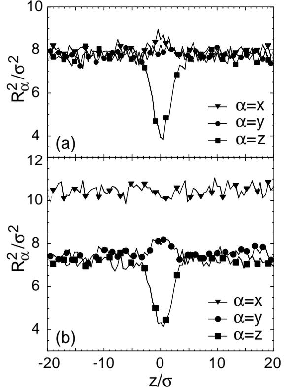
FIG. 5. The mean square components of the end-to-end distance along  $\alpha = x, y$ , and  $z$  as a function of the center of mass height  $z$  for  $N = 16$  polymers with  $\epsilon^* = 3.2$  at (a)  $v_W = 0.1\sigma/\tau$  and (b)  $v_W = 0.5\sigma/\tau$ . Although the viscosities at both shear rates are nearly indistinguishable from the limiting Newtonian viscosity, there is a clear stretching of polymers along the flow direction in (b).
